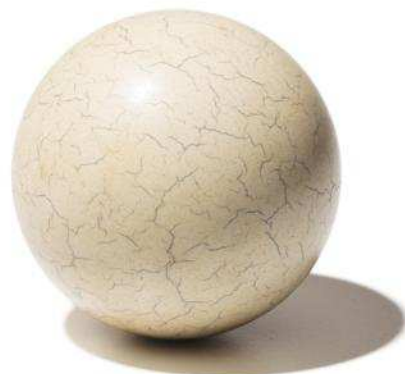
This 19th-century billiard ball was made from celluloid, an early plastic that replaced elephant ivory—which was already growing scarce.
