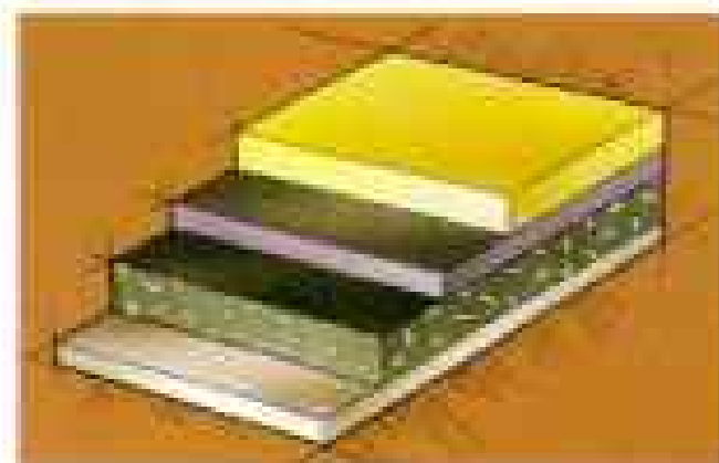
Sound-dampening asphalt and steel sheets are sandwiched together to help minimize vibration and noise.
