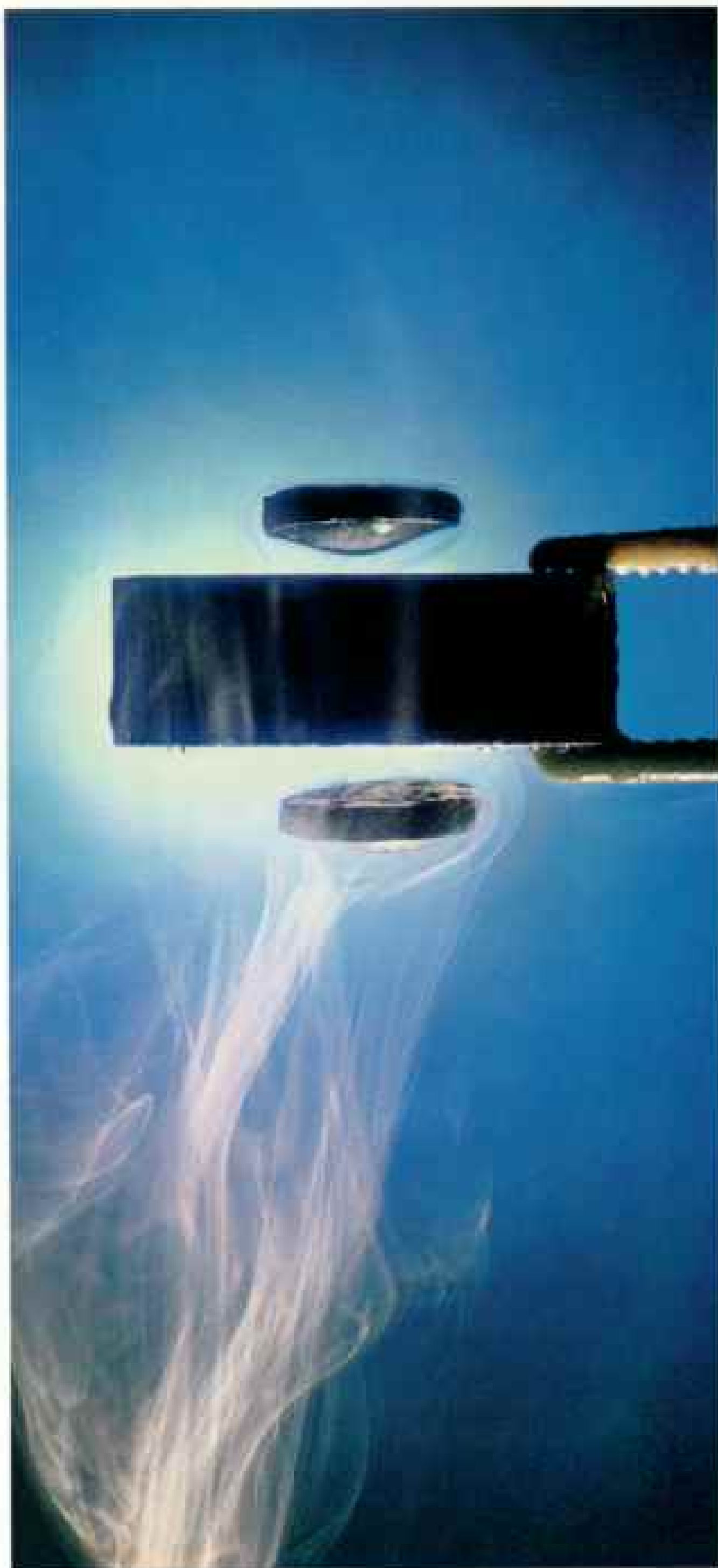
Wisps of vapor from frigid nitrogen envelop a thallium-based superconductor at the University of Arkansas. This superconductor has a rare characteristic: the ability to suspend magnets both above and below it. Possible applications include ball bearings that operate with no friction.
