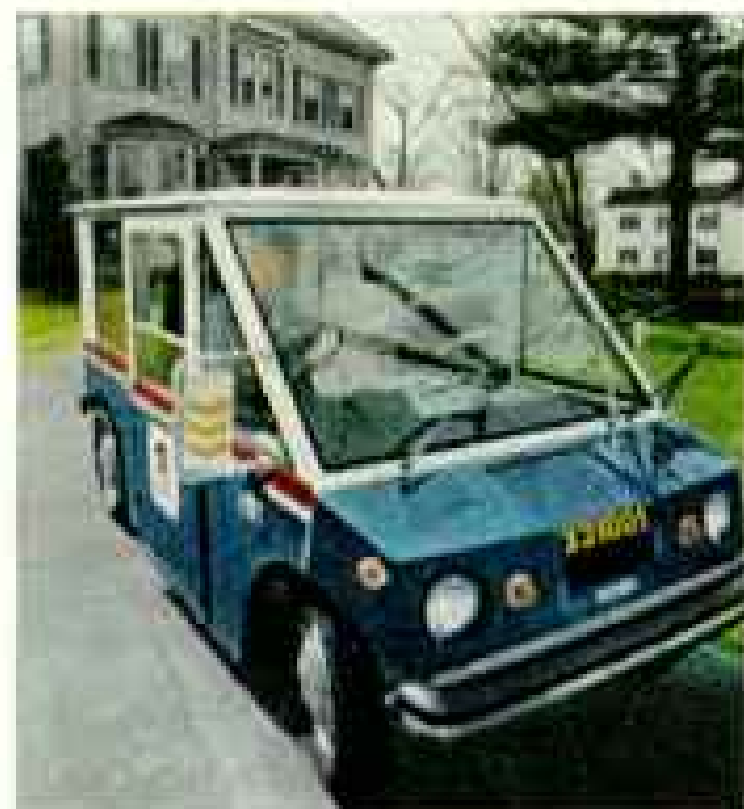
Improved lead-acid batteries make electric-powered vans practical for urban delivery. The next step—practical battery-powered cars.
