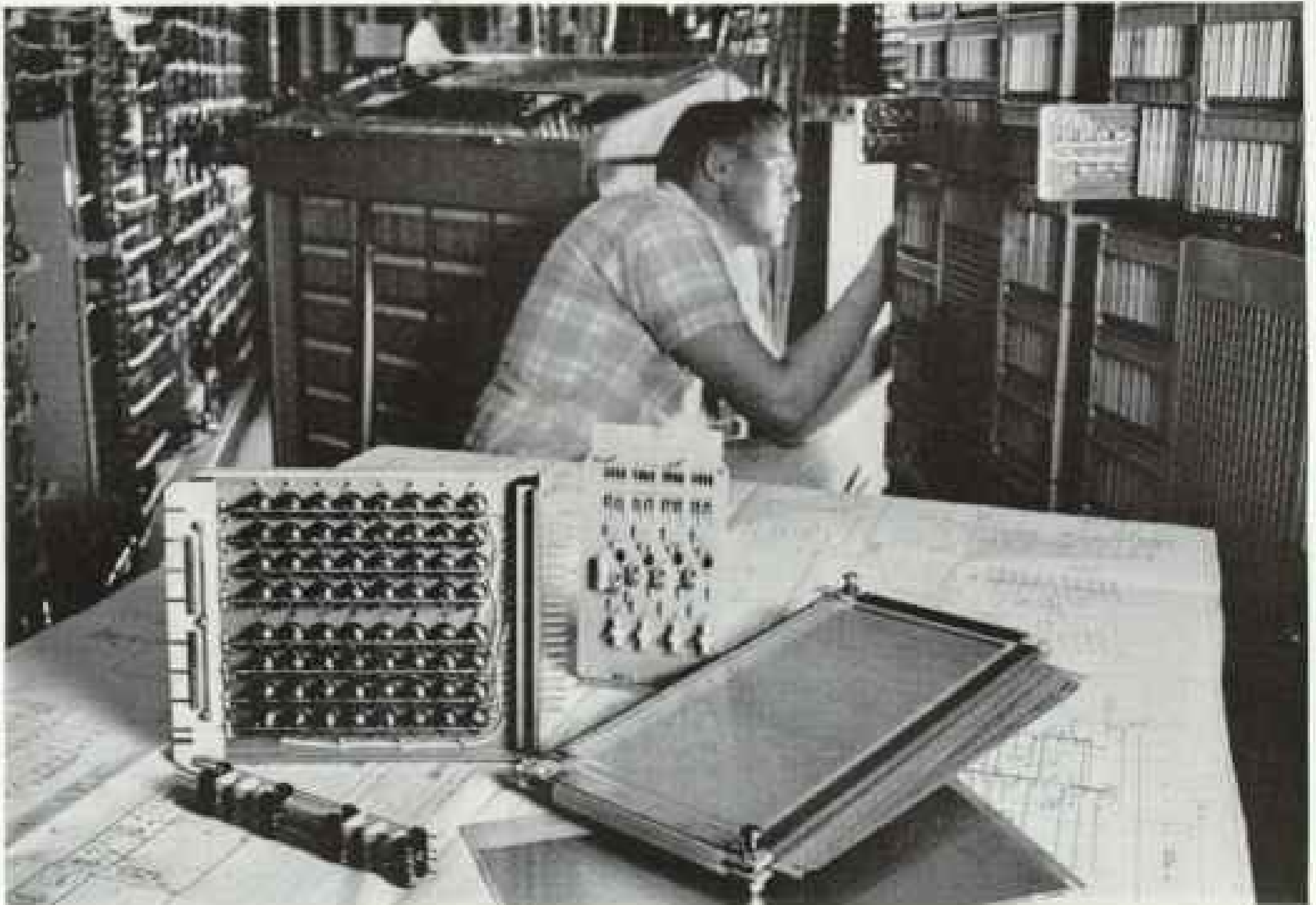
CENTRAL CONTROL SECTION that handles logic and command functions for ESS is shown in background. Foreground shows basic components.
