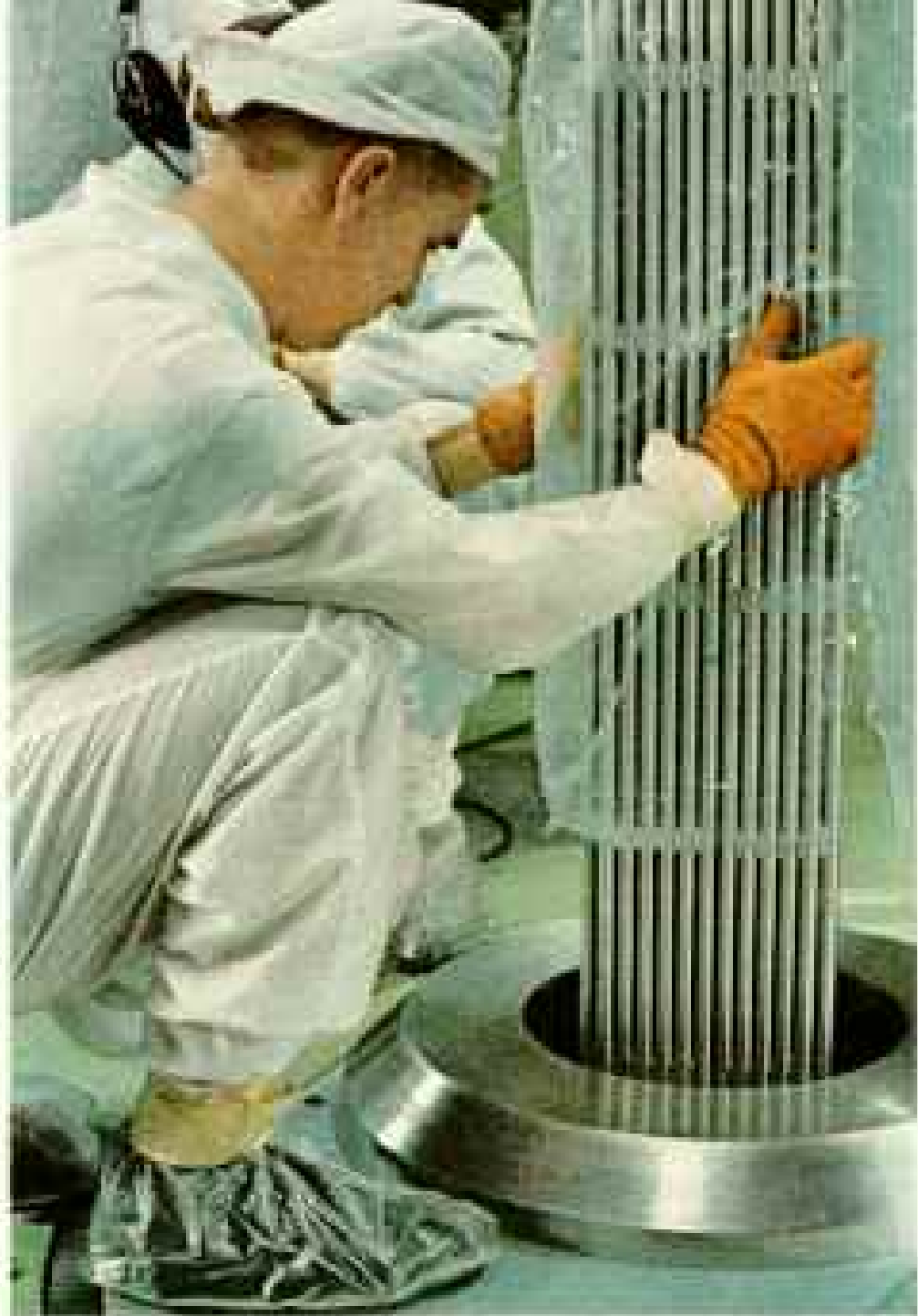
Shedding its sheath of protective plastic, a fuel element of steel tubes containing uranium pellets slides into the reactor.
