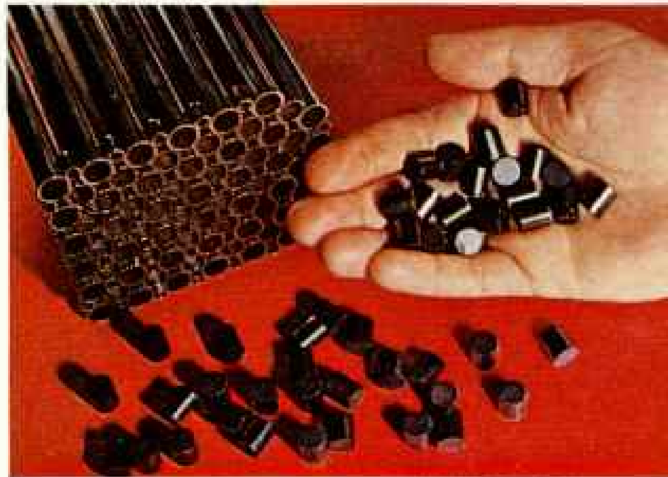
Potent pellets of uranium oxide do the work of coal or oil. Loaded into steel tubes, 815,440 slug-pack enough power to drive the ship 300,000 miles. Until activated, they offer no radiation hazard.
