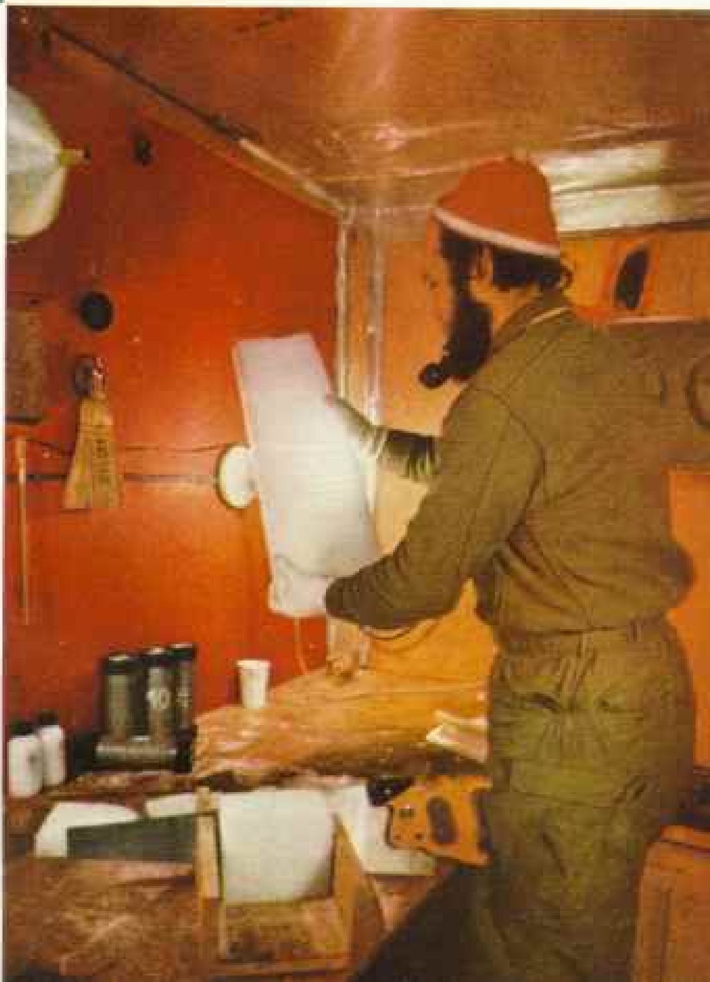
History locked in ice: As a tree's rings tell its past, so layers of snow and ice reveal the icecap's. In his workshop, glaciologist E. W. Remington slices blocks of snow with saw and miter box and examines them under light. After laboring in the snow mine, he "warms up" in this room, where temperatures hold around 25 below.
