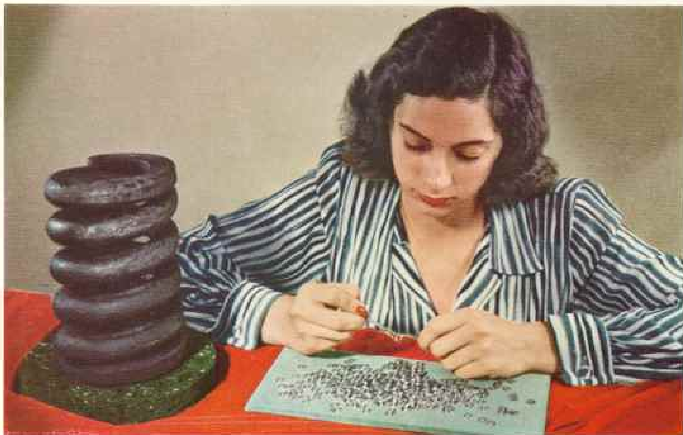
Rugged Car Spring and Delicate Watch Springs Cushion and Time Trains with Steel If made of proper alloy, a 22½-pound car spring, valued at $1.38, would produce 225,000 hairsprings worth $400,000. Drawing to fine gauge would stretch it to 43 miles. This Hamilton Watch employee sorts 517 hairsprings.
