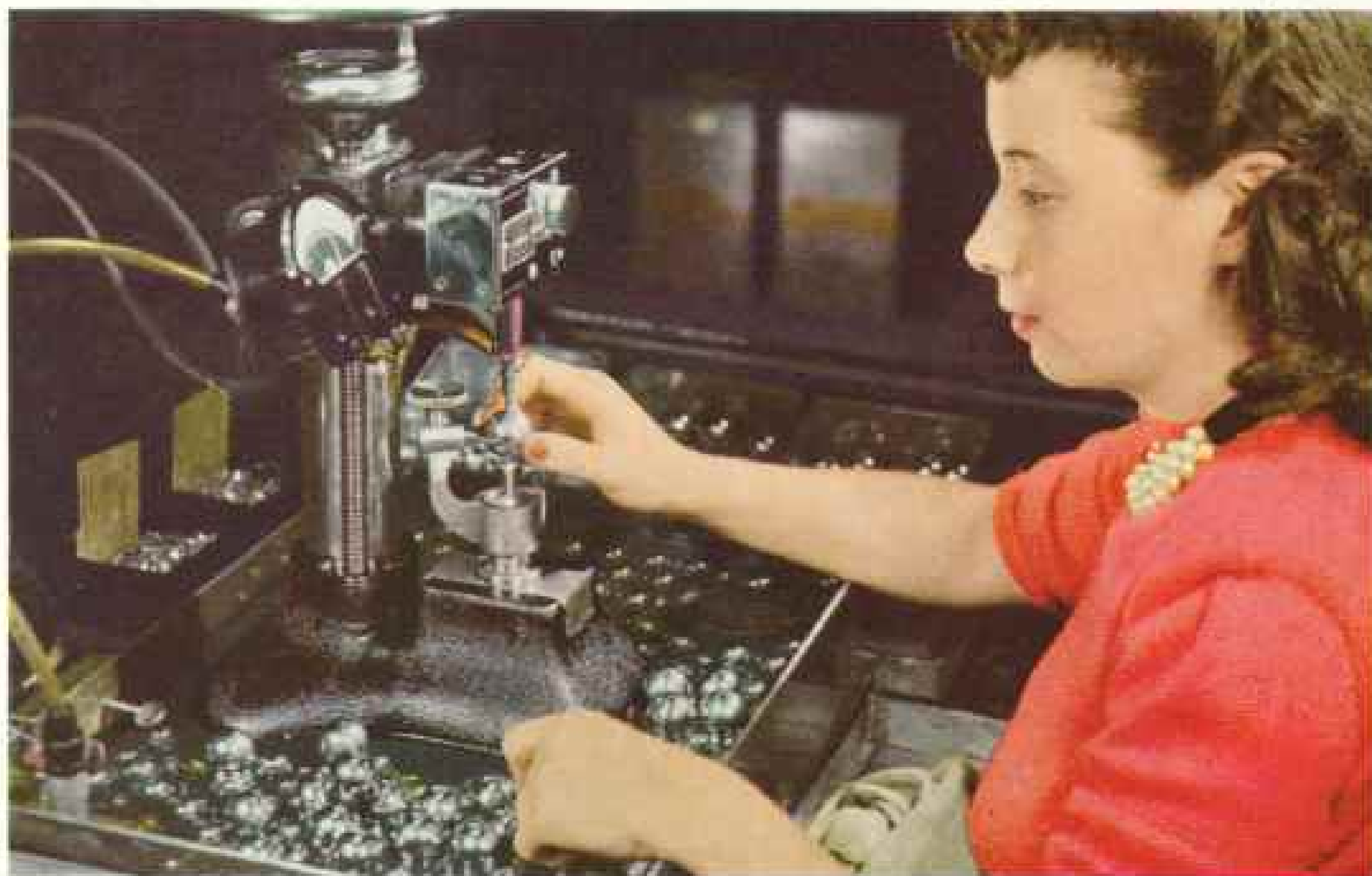
Rugged Car Spring and Delicate Watch Springs Cushion and Time Trains with Steel If made of proper alloy, a 22½-pound car spring, valued at $1.38, would produce 225,000 hairsprings worth $400,000. Drawing to fine gauge would stretch it to 43 miles. This Hamilton Watch employee sorts 517 hairsprings.
