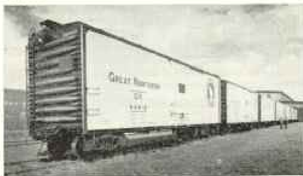
Great Northern pioneered quantity construction of plywood-steel freight cars. Light, but sturdy, these cars are ideal for grain, forest products and merchandise.
