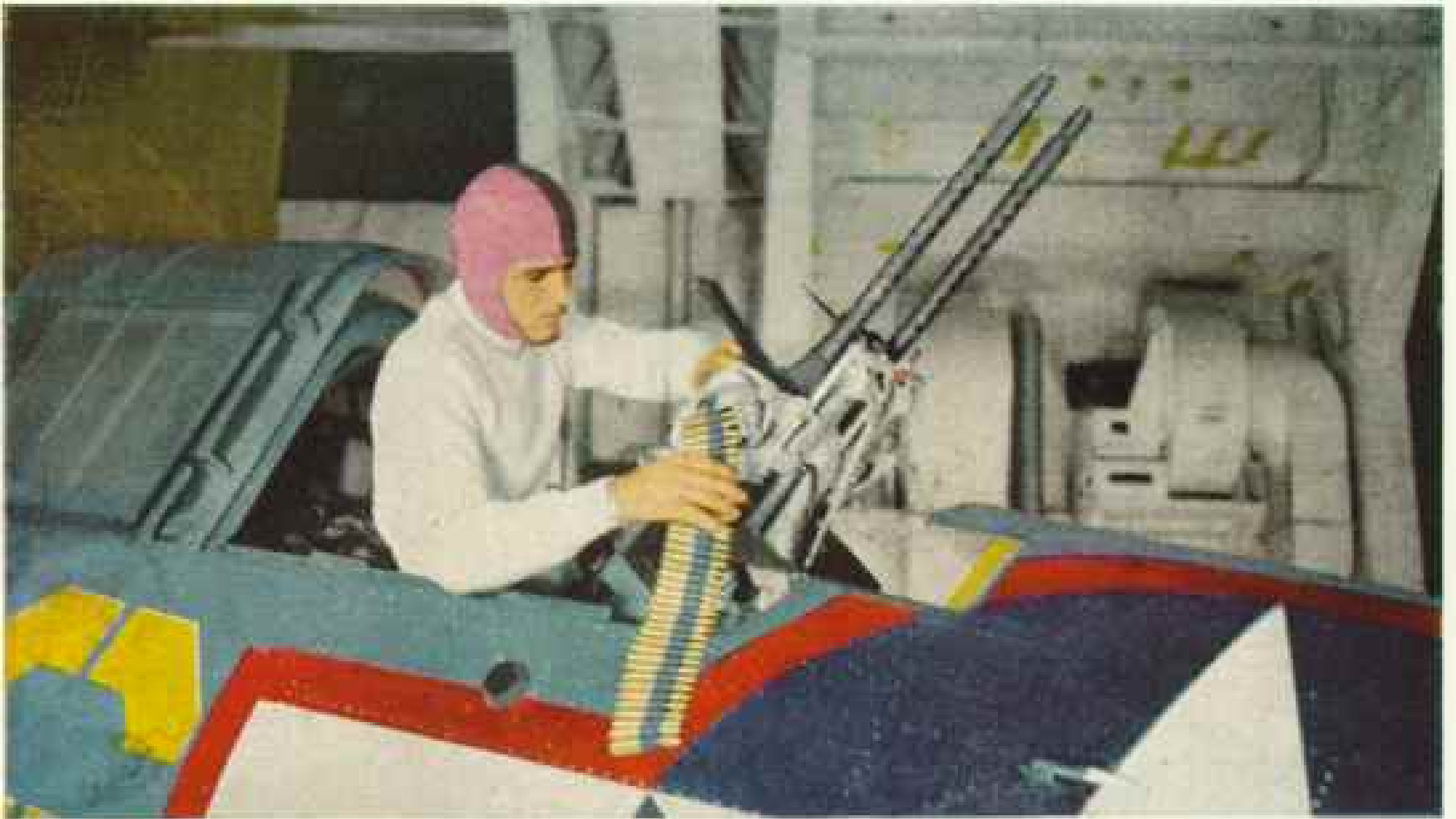
Ordnanceman Checks Twin 30s of a Scout Plane on the Hangar Deck
