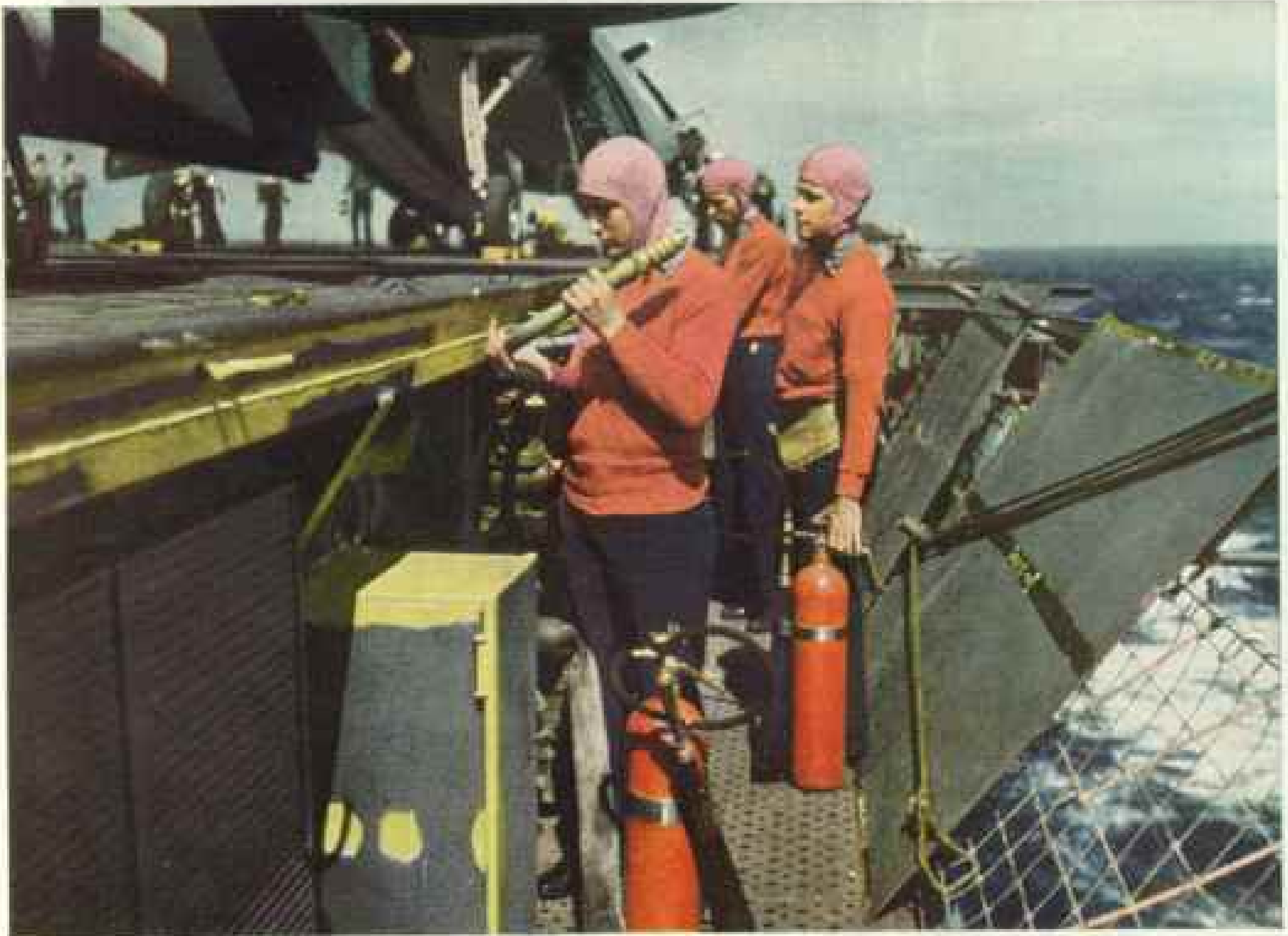
Using Fog Sprays and Extinguishers, Red-clad Fire Fighters Can Snuff Out Infernos. Behind curtains of water from the nozzles, they advance close to gas flames, smothering them with fine mist. Because flattops carry vast stores of gas and bombs, they are elaborately equipped for fire fighting.
