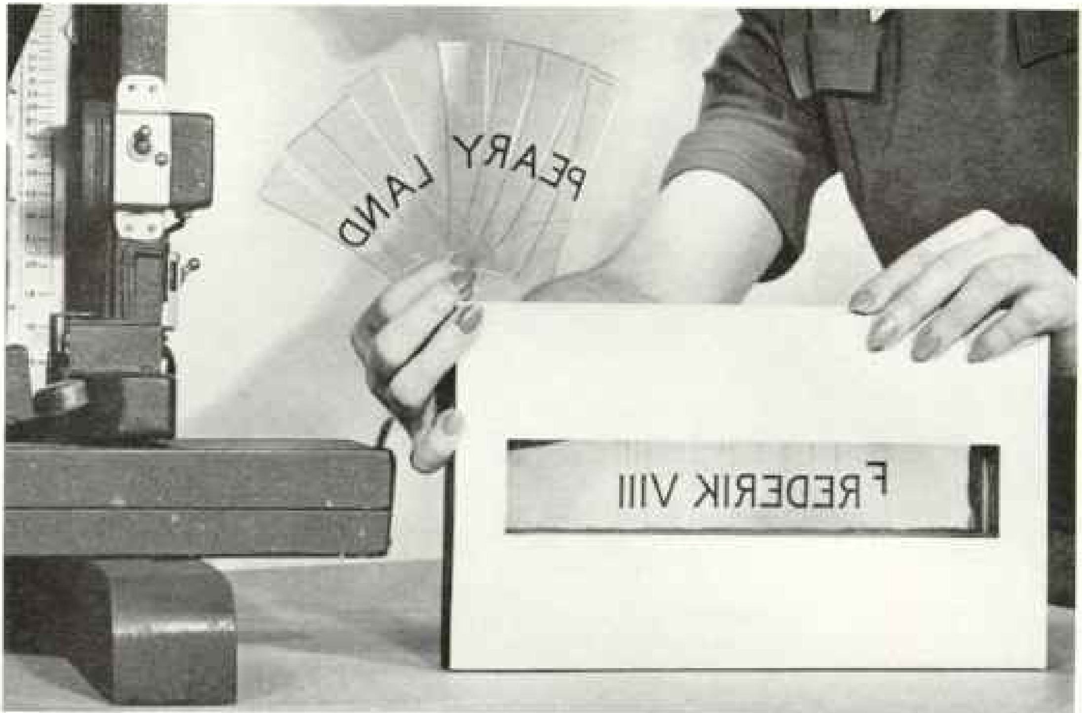
For One Man to Letter a Whole Map Would Be Slow, and Letters Would Lack Uniformity So an expert draws the alphabet and each letter is photographed. Transparent film positives are set like type (above) and the name is printed. The late A. H. Bumstead and his son developed the method.
