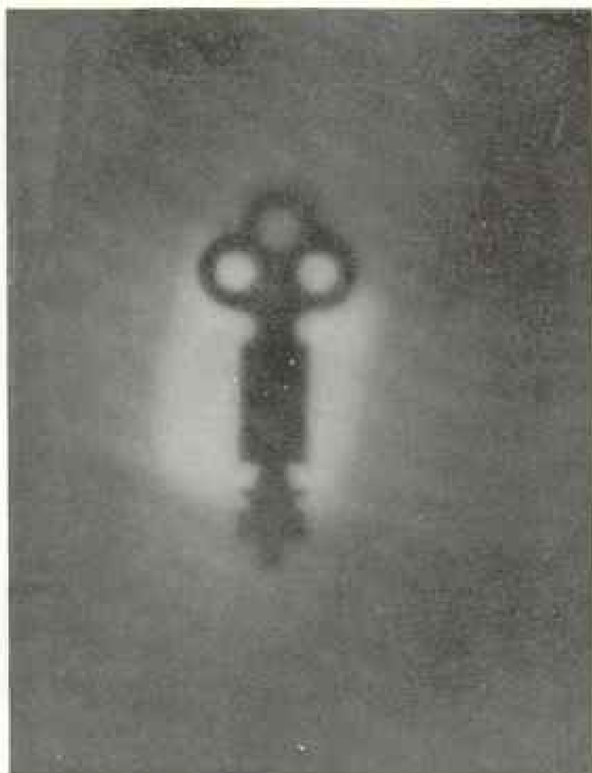
A RADIOGRAPH OF A KEY
