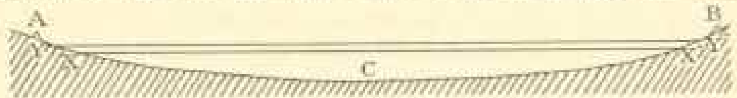
FIG. 6—DIAGRAM ILLUSTRATING THE METHOD OF USING A LAKE SURFACE FOR THE DISCOVERY AND MEASUREMENT OF EARTH MOVEMENTS
