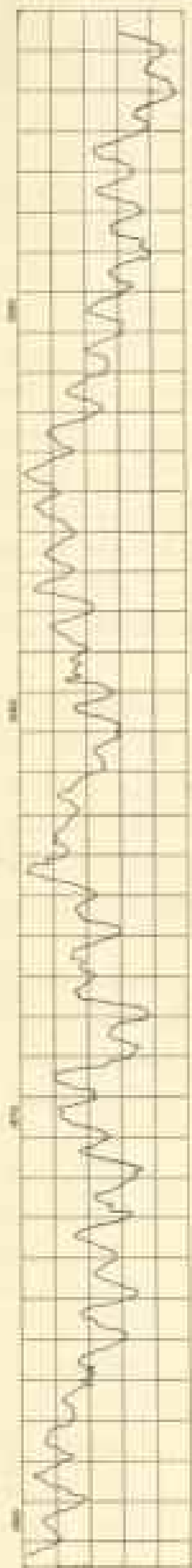
FIG. 4.—ANNUAL OSCILLATIONS OF THE SURFACES OF THE LAURENTIAN LAKES Computed from monthly means published by the Chief of Engineers, U. S. A. Each vertical space represents six inches. The observations for Lake Superior cover the period 1862-1891; for Michigan-Huron, 1860-1891; for Erie, 1855-1891; for Ontario, 1850-1891.
