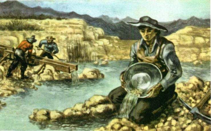
Mining gold with sluice and pan.
