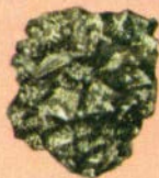
Uneven fracture: arsenopyrite
