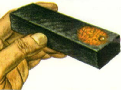
Blowpipe test for zinc: heating ore on charcoal with oxidizing flame.
