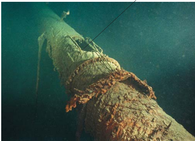
FALLEN FOREMAST Although severely damaged, the crow's nest is clearly visible on the fallen foremast. From this vantage point, two lookouts kept watch around the clock for icebergs, ships, and other hazards.
