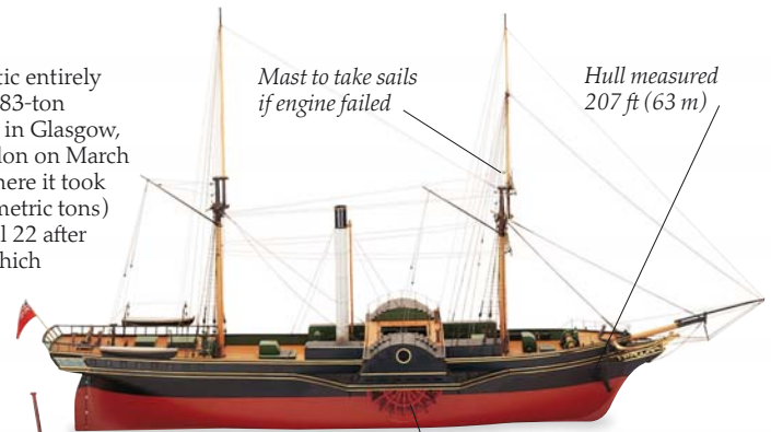
Paddle wheels driven by steam engine
