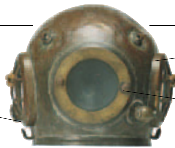
Helmet equipped with two-way communication system so diver can talk to someone on the surface
