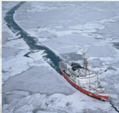
Ice breakers have thick steel hulls to crush ice and open up a lane for other ships
