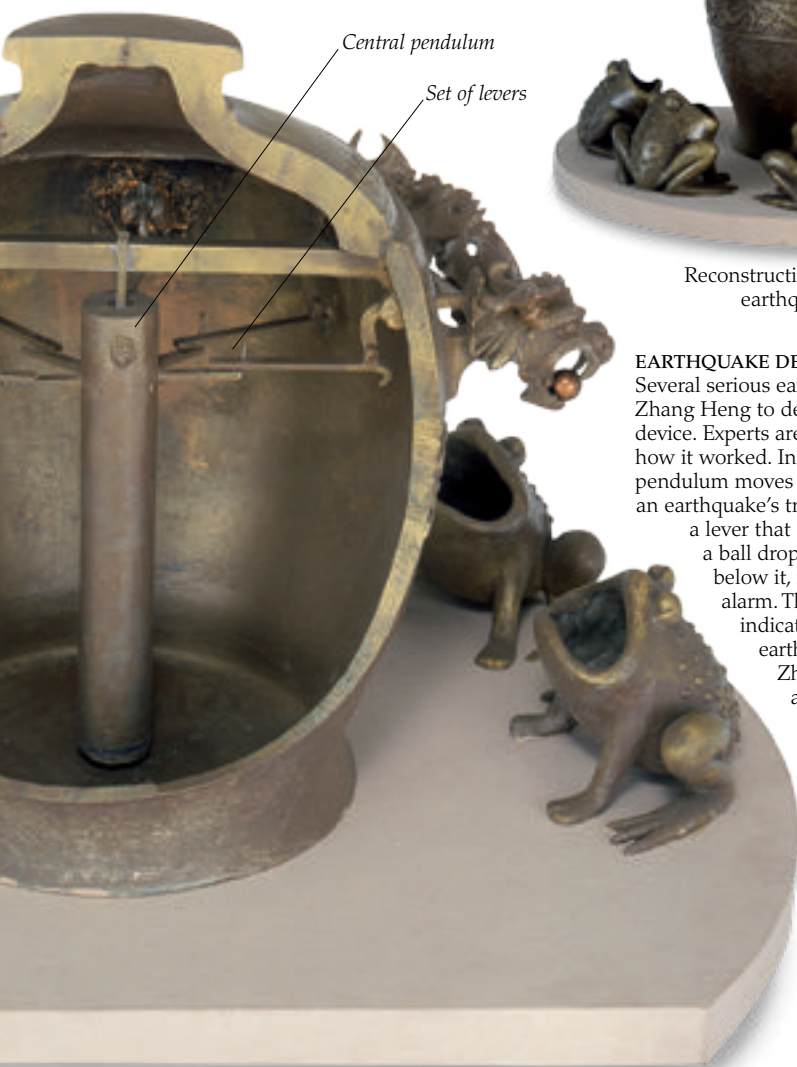
Cross-section of Zhang Heng's earthquake detector
