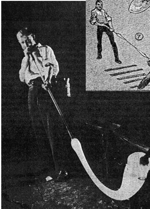
Figure 7 Glassmaking. Powell's Glass Works, London. The processes of glass manufacture: 1-5, Making Flint glass for windows; 6. Melting-pot for Flint glass; 7. Making glass tubing
