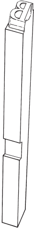
4 Gutenberg's breakthrough – a piece of movable type (actual length 23 mm). The little nick on the side allowed the compositor to tell, by touch alone, which side was up. The reversed image of a capital B forms the upper surface.
