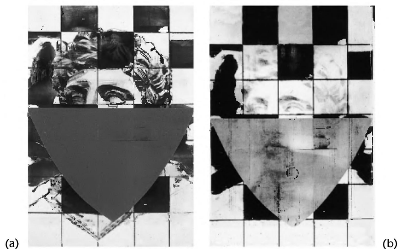
Fig. 7.7a,b. (a) Painting of a head partially obscured by a grid and checkerboard in blue and a red shape. The head is painted in raw umber containing manganese, overlain by grid lines and squares painted in cobalt blue. The red shape is painted in cadmium red. (b) First autoradiograph of the painting produced by beta radiation emitted by the isotope cobalt 60m. Exposure is for 10 minutes, beginning 15 minutes after activation. (Continued on pg. 85.)
