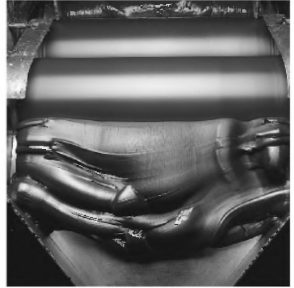
Fig. 2.4. A modern commercial three-roll mill producing, in this case, permanent green oil paint (Courtesy, Daniel Smith Artists' Materials.)
