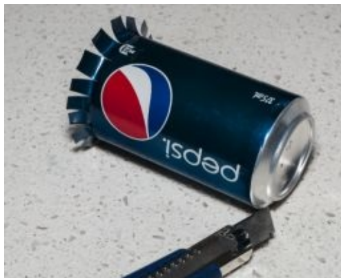
Image 50 - Use a Box Cutter to Open the Bottom of the Can
