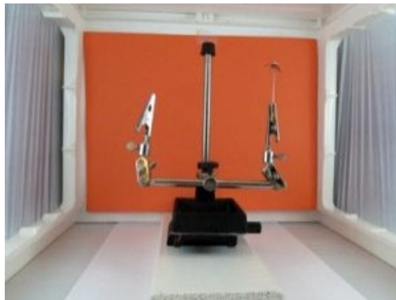
Image 86 - Focus stacking setup
