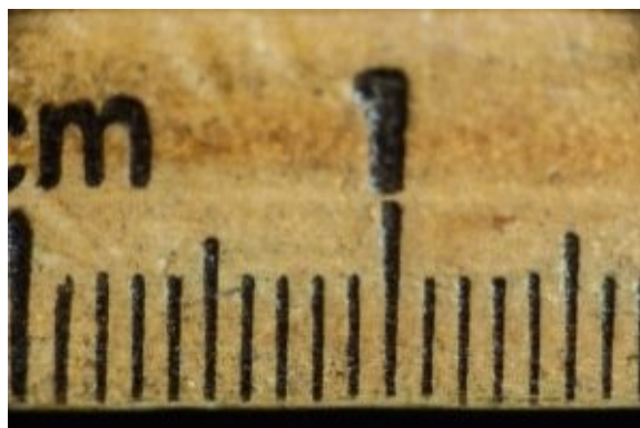
Image 4 - Photograph of a ruler with a macro lens + 68mm extension tubes. Approximately 17mm in length.
