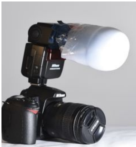
Image 52 - DIY Flash Diffuser
