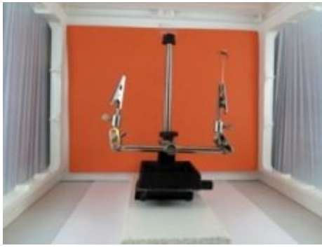
Image 83 - Focus stacking and specimen holder setup
