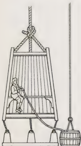
▲ Dr Edmund Halley's diving bell of 1690 was the first bell in which divers were not restricted to the amount of air contained in the vessel itself. Halley's bell was supplied with air through a leather pipe leading from a weighted, air-filled barrel. As one barrel was exhausted, another was lowered from the surface to replace it.
