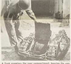
A Yank examines the rear compartment, housing the control wire, of a German remote-controlled military tank. The remote-controlled, called the "doodlebug" by the Allies, was knocked out by machine gun fire in Italy.
