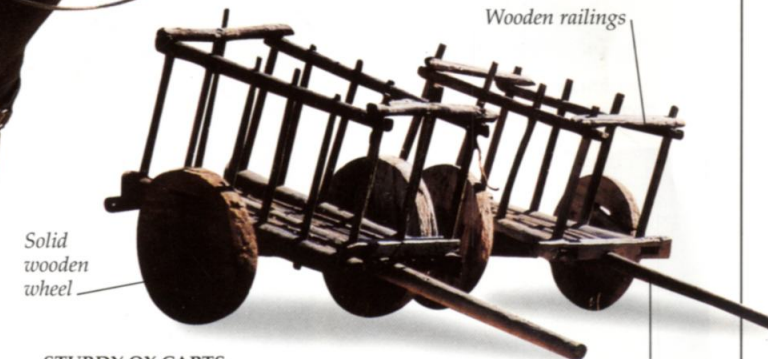
STURDY OX CARTS The dependable ox was the favored draft animal in most of the Spanish Southwest, and these wooden-wheeled carts were the most common vehicles in use. The cart required a span of two oxen; the driver walked alongside cracking a whip or switch to control the team.
