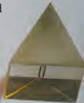
A refracting glass prism disperses white light into its component colors.
