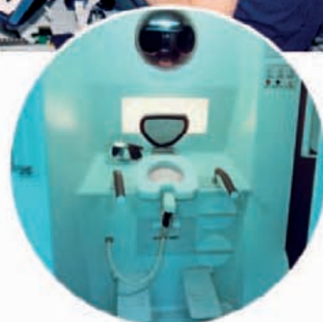
▲ SITTING COMFORTABLY Astronauts strap themselves onto toilets that use suction to remove waste. On early missions, astronauts collected their waste in hoses and plastic bags.
