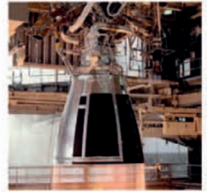
▲ TESTING The RS-68 rocket has liquid-fuel engines. Its exhaust gases are nearly transparent.
