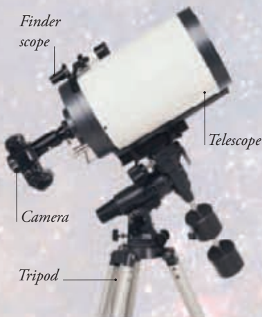
▲ LONG SHOT Pictures of very faint objects can be taken by attaching a camera to a telescope and leaving the shutter open for at least half an hour.
