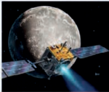
The European Space Agency's SMART-1 lunar probe is powered by an ion drive.
