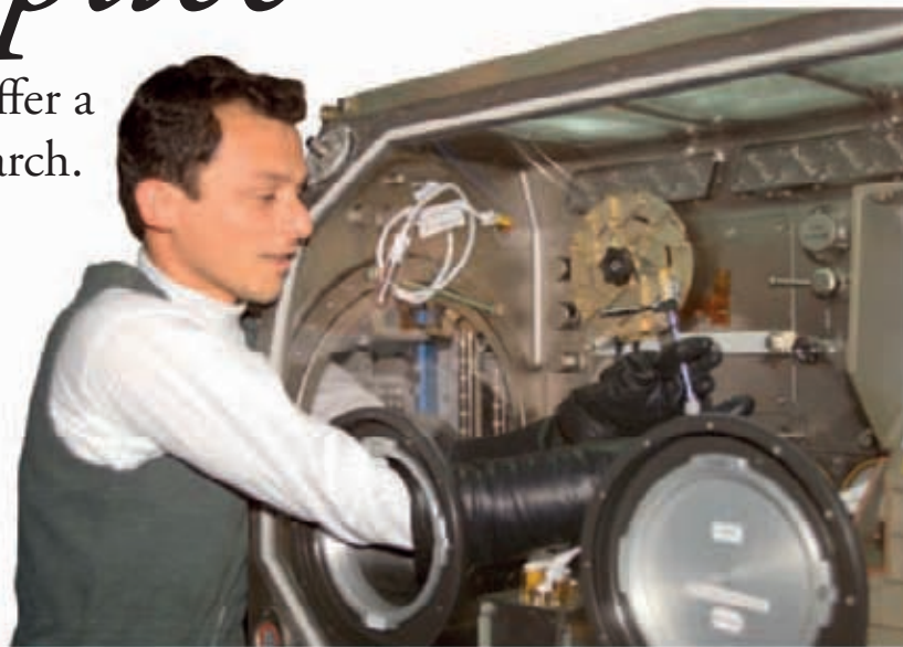
▲ GLOVE BOX EXPERIMENTS Astronauts study the effects of zero gravity in the Destiny laboratory on the ISS. A glove box provides a safe, enclosed area for experiments.
