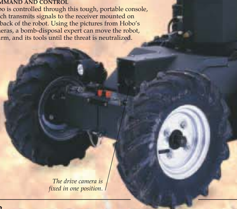
Hobo's low centre of gravity enables it to balance at steep angles.
