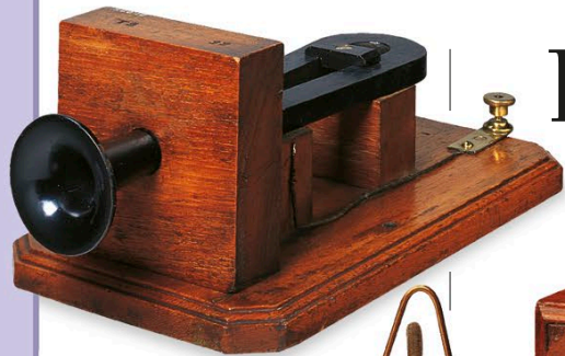
Bell's box telephone incorporated a larger magnet than others, which made it more sensitive.
