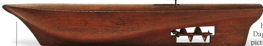
SHIP'S PROPELLER This is a model of SS Francis Smith, which was fitted with Smith's propeller. Modern ships have their propeller further back.
