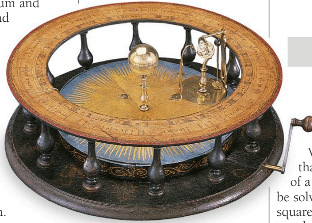
SOLAR SYSTEM Users turned the handle of this 18th-century orrery to show the annual rotation of the Earth around the sun and the moon's rotation around Earth.
