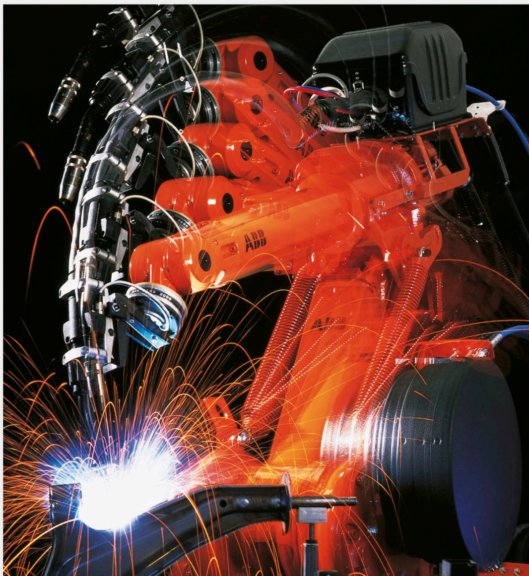
A robot arm spot-welding the suspension unit of a car. Robots are ideal for dangerous, repetitive jobs like this.
