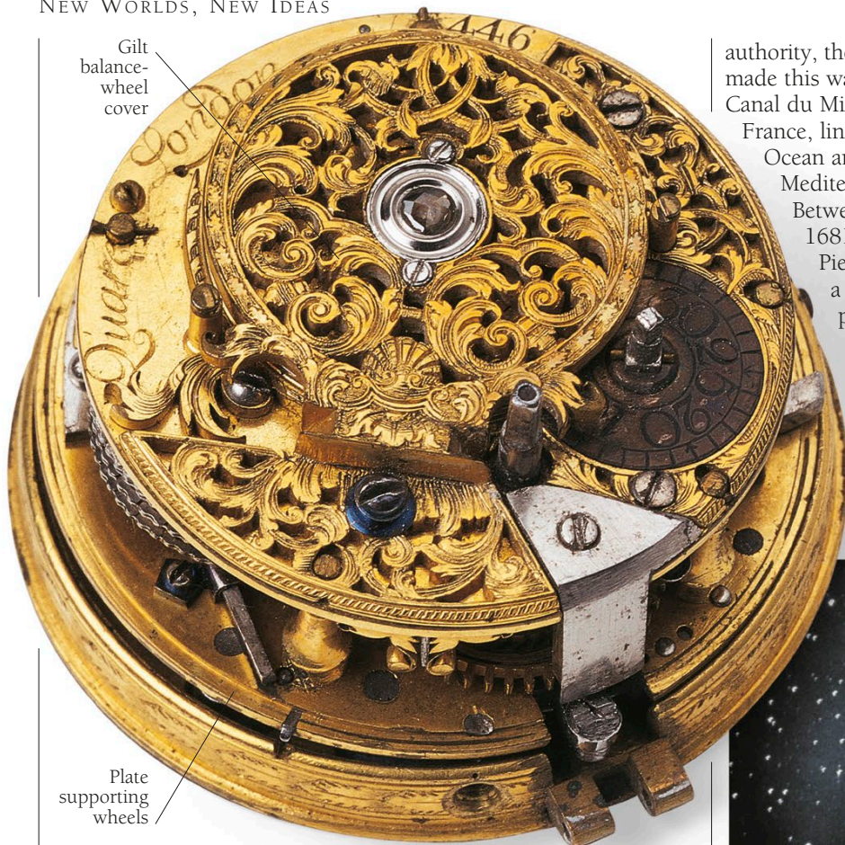
REPEATING WATCH The exquisite mechanism of this Quare repeating watch was normally hidden from its user.
