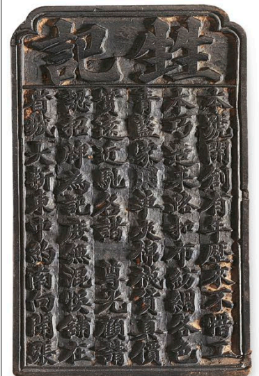
BLOCK PRINTED BOOK Patterns and symbols are carved into this wooden printing block.
