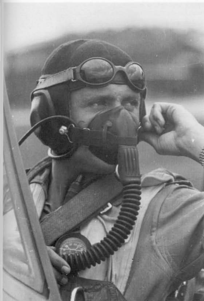
Above: The type of oxygen mask worn with the net flying helmet.
