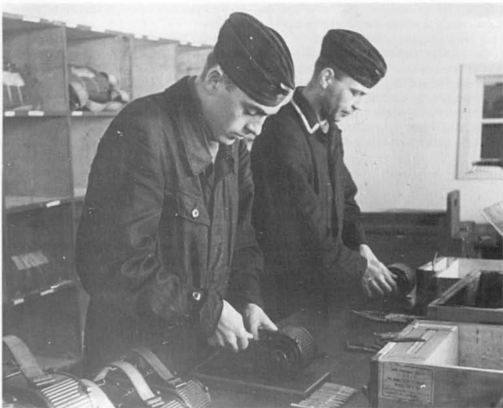
Left: Two armourers, both wearing the one-piece black fatigue overalls, load machine-gun ammunition into saddle and cylinder drums. The man in the background, being an NCO, wears braiding around his collar.
