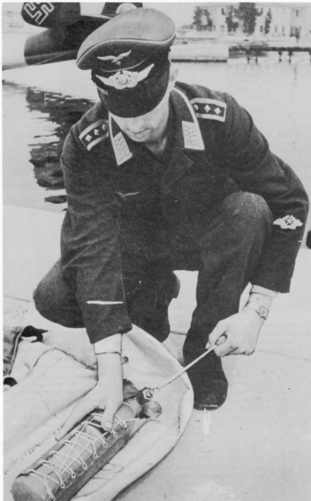
Left: An Oberfeldwebel inspecting and testing the compressed-air bottle for inflating a rubber dingy. The trade badge on his left forearm is that for Flieger-technisches Personal.
