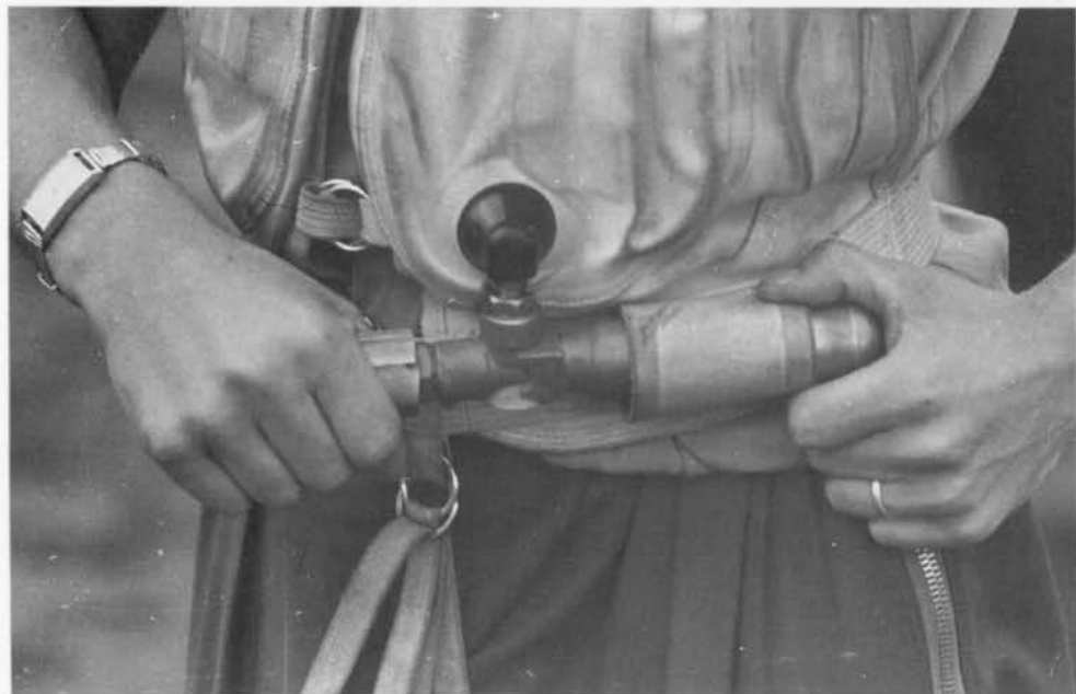
Left: A close-up of the cylinder of compressed air used to inflate the life jacket.
