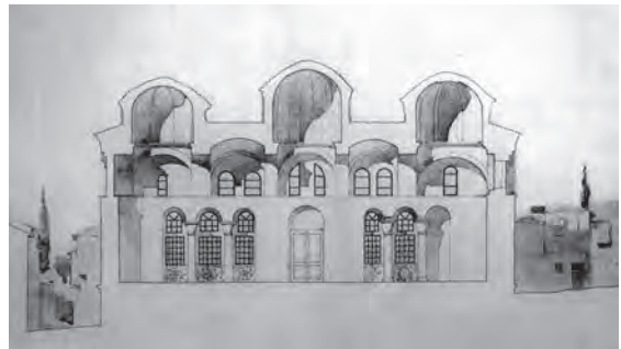
405. St Theodore, Constantinople. Longitudinal section through the outer narthex with its three domes, looking west at the entrance door in the centre and the flanking external windows
