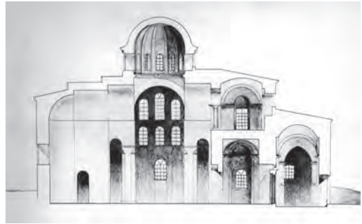
398. St Saviour Pantepoptes, Constantinople. Cross section through apse (left), central dome (centre) and two narthexes (right)
