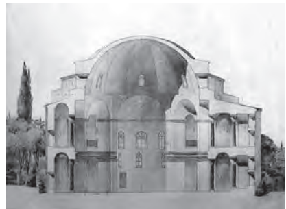
431. SS Sergius and Bacchus, Constantinople. Section through apse (left), naos and dome (centre) and narthex (right)
