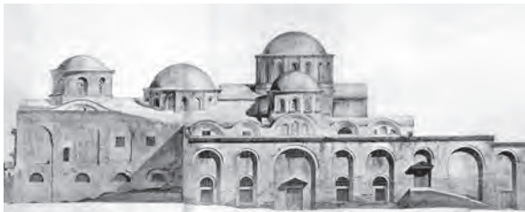
420. St Saviour Pantokrator, Constantinople. Arched entrance façade of the outer narthex (foreground), small dome over the inner narthex, large dome over the south church (right), lower dome of the middle church (centre) and dome of the North church (left)
