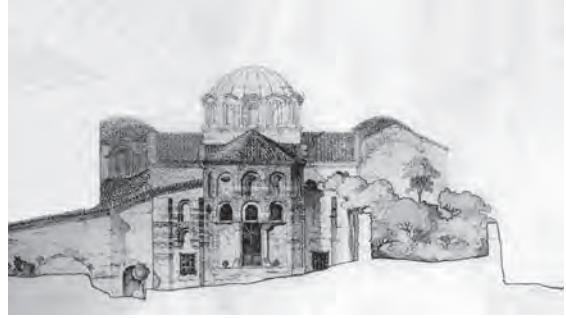
403. St Theodore, Constantinople. East façade with the triple windows of the bema apse
