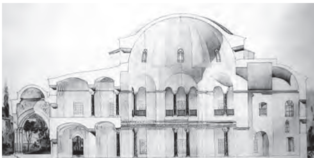
432. SS Sergius and Bacchus, Constantinople. Section through Ottoman portico (left), naos and dome (centre) and apse (right)
