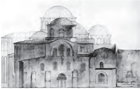
422. St Saviour Pantokrator, Constantinople. North elevation showing side entrance into north church (centre), narthex (right wide arch window) and outer narthex further back (far right)
