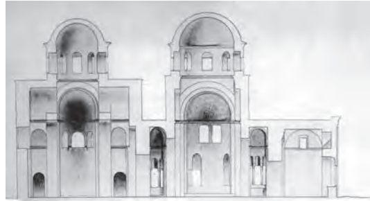
380. Theotokos Panachrantos, Constantinople. North-south section through the two Churches (left) and the parekklesion (right)
