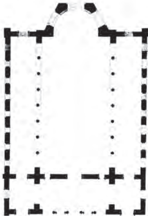
127. Basilica plan type – St John Studios, Constantinople. Narthex (bottom), side aisles and projecting bema apse
