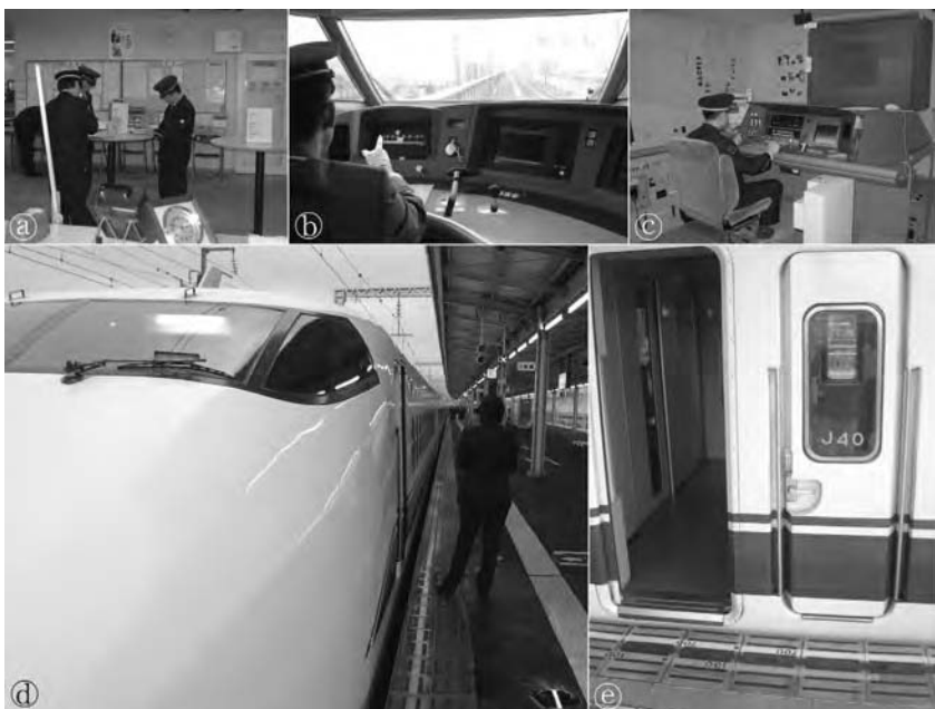
Figure 6.4 (a) Having checked their clocks against the ‘standard’ in the foreground, the crew confirm their orders for their next journey. (b) A driver confirms that he has acknowledged the change in ATC limit on an E2-series shinkansen. (c) A new JR Tōkai recruit practices on a shinkansen simulator. (d) The conductor checks along the platform that there are no problems. (e) Marks on the platform show where the train should stop – the dot in between the numbers relating to the series of shinkansen should be in the middle of the cab door, as in this case.
