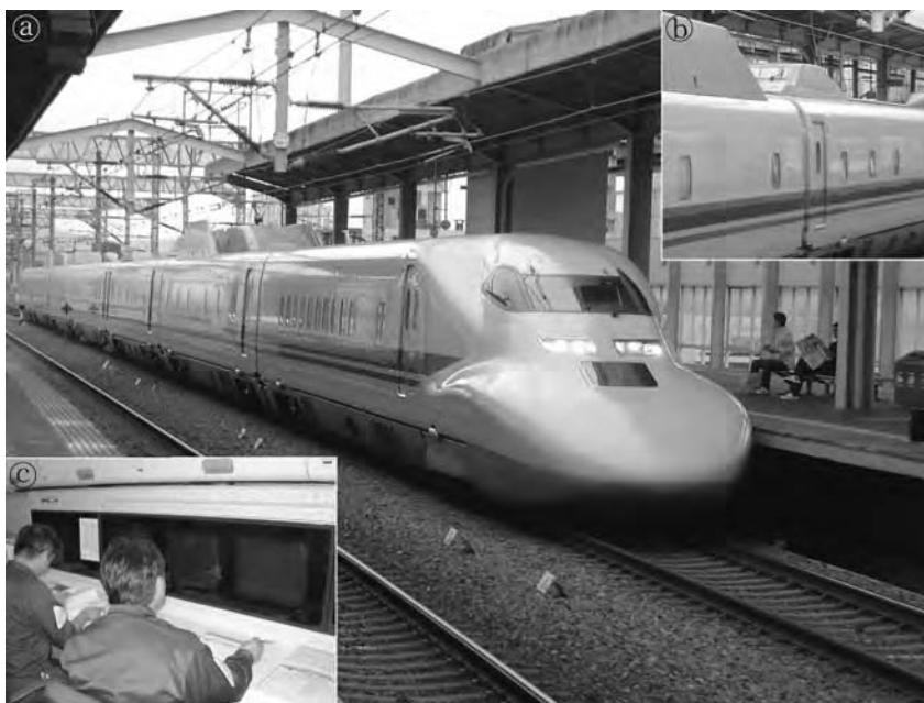
Figure 6.1 (a) The T4 Dr Yellow at Kokura station – a video camera for recording the track is visible in the area beneath the headlights; (b) viewing points in the roof of the train allow first-hand observations of the connection between the pantograph and overhead power cables – a live video feed is also provided to a screen in one of the carriages; (c) staff monitoring information on board Dr Yellow.
