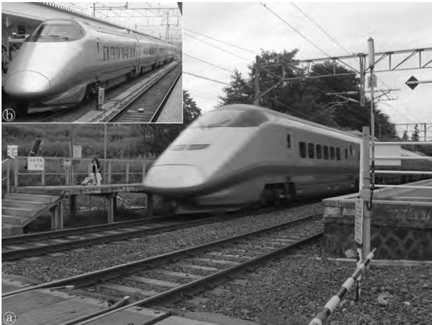
Figure 5.3 (a) An E3-series shinkansen passing a level crossing and station served by wide-gauge-conventional trains along the Yamagata Shinkansen; (b) a 400-series shinkansen at Yamagata station.
