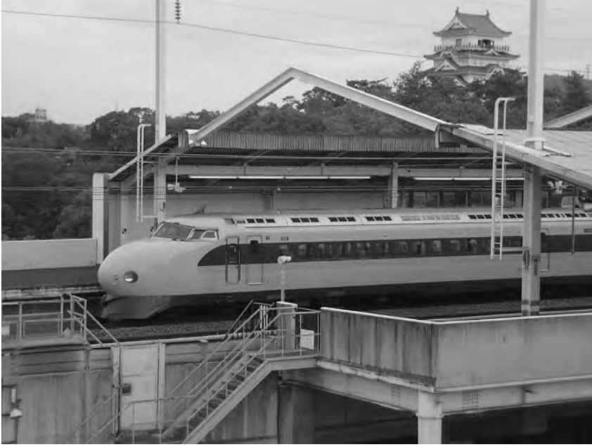
Figure 3.1 The familiar rounded ‘bullet’ shape front of the original shinkansen – here in its ‘renewal’ design – at Fukuyama station, with Fukuyama Castle in the background.
