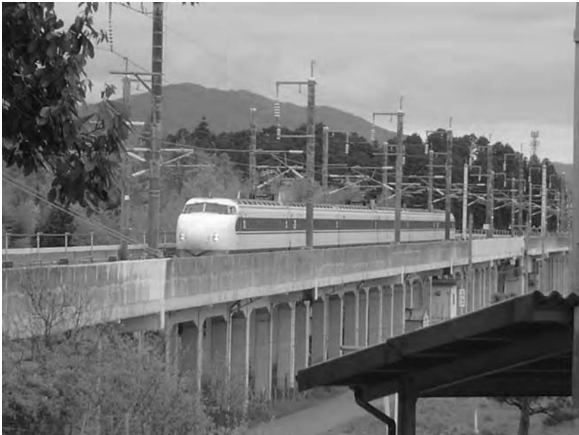
Figure 2.7 A 0-series shinkansen near Higashi-Hiroshima. Note how although this service is only 6 carriages long rather than 16 as in the past, it has more pantographs (three) than are found on newer shinkansen.
