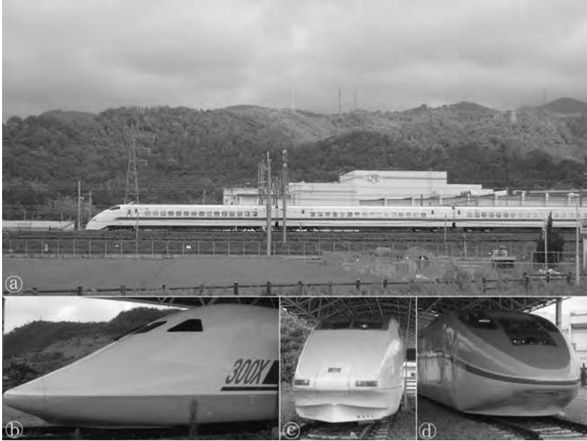
Figure 5.11 (a) A 300-series passing the RTRI large-scale low-noise wind tunnel facility in Maibara, outside of which three experimental trains are housed; (b) 300X; (c) STAR 21; (d) WIN350.
