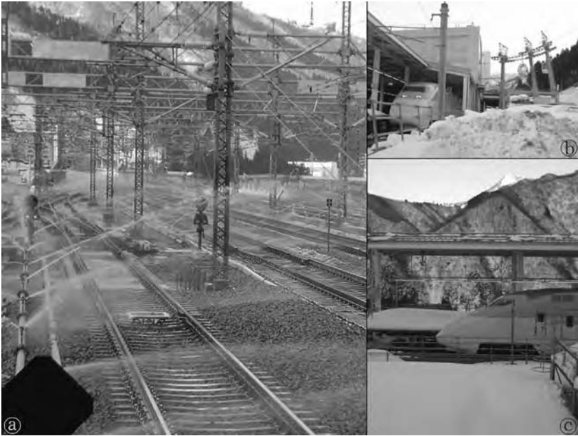
Figure 7.2 (a) Sprinklers in action at Echigo-Yuzawa – note how the main line appears to disappear into a river in the distance; (b) An E1-series shinkansen at Gāla-Yuzawa station, where gondolas take passengers direct from the station to the ski slopes; (c) An E1-series shinkansen at Gāla-Yuzawa station with the impressive mountains of the region in the background.
