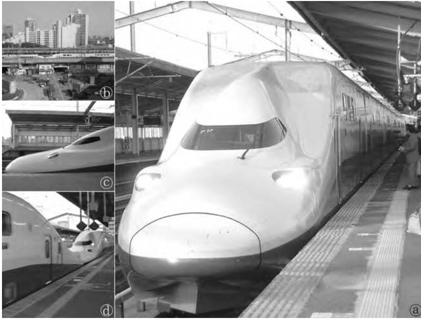
Figure 5.8 (a) A double-decker E4-series arriving at the popular commuter city of Utsunomiya; (b) an E4-series linked with a 400-series passing Kita-Yono station in Saitama – note how the windows on the lower deck of the E4-series are almost totally obscured by the sound-protection wall in this area where there was much opposition to the construction of the shinkansen line; (c) the E4-series in profile reveals some of its links to the 700-series design; (d) two E4-series shinkansen joined together – the highest capacity high-speed train service in the world.
