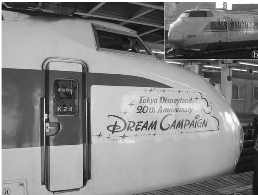
Figure 6.8 (a) A 200-series shinkansen during the campaign promoting Tōkyō Disneyland; (b) a 200-2000-series shinkansen, which was based on the 100-series design rather than the 0-series design as used for the 200-series.
