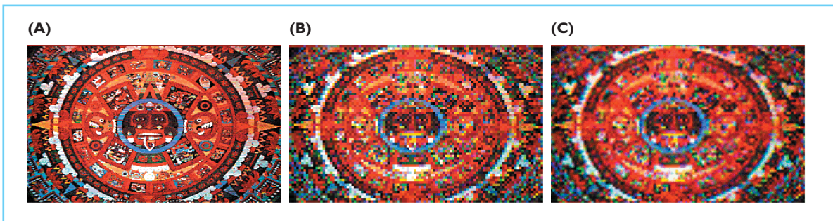
Figure 8.6 Spatial artifacts caused by demosaicing algorithms. The original image is shown in (A). Interpolation errors when using (B) linear interpolation and (C) pixel replication are shown.
