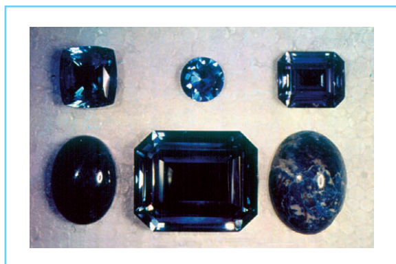
Figure 7.1 Six blue gemstones with different causes of color. (Left to right, above) Maxixe-type beryl (radiation-induced color center), blue spinel (ligand field color from a cobalt impurity), spinel ‘doublet’ (colorless spinel containing a layer of organic dye); (below) shattuckite (ligand field in an idiochromatic copper compound), blue sapphire (Fe-Ti intervalence charge transfer), lapis lazuli ( S_3 anion-anion charge transfer); the largest stone is 2 cm across.
