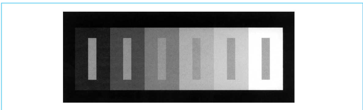
Figure 4.14 Example of achromatic contrast. All of the vertical stripes are physically identical but they appear different because of the light level in the surrounds.
