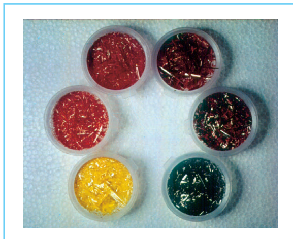
Figure 7.29 Mixed solid solution crystals of yellow cadmium sulfide CdS and black cadmium selenide CdSe showing the intermediate band-gap colors as in Figure 7.27.
