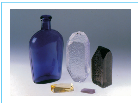
Figure 7.33 (Left to right, above) century-old glass bottle, irradiated to form 'desert amethyst glass' (color center); colorless synthetic quartz crystal as grown, and one that has been irradiated to form smoky quartz (color center); below: a synthetic citrine quartz colored yellow by Fe (transition metal impurity) and one that has been additionally irradiated to form amethyst (color center).
