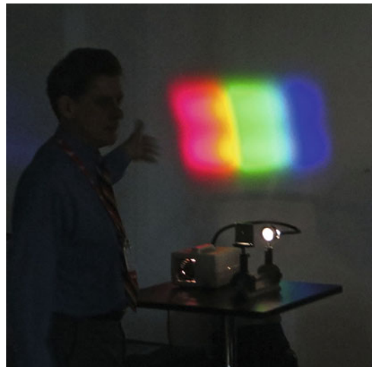
Color Circle, Fig. 3 Lindsay MacDonald demonstrating how a prism separates white light into different colors
