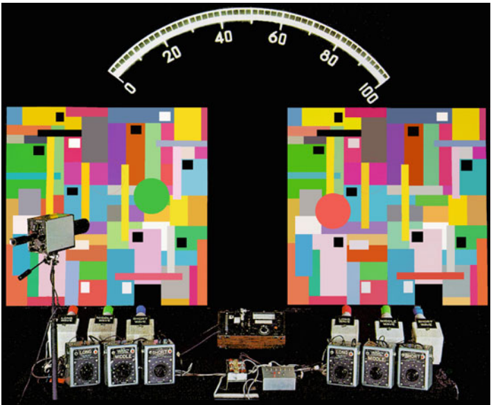
Retinex Theory, Fig. 2 Land’s double Mondrian experiment. Two identical sets of matte colored papers, with separate L, M, S illuminating projectors with voltage transformers for control of the amount of light. Telephotometer readings were projected above the Mondrians. The
