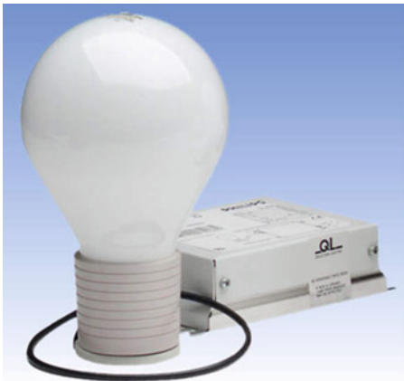
Induction Lamp, Fig. 4 Pear-shaped induction lamp with internal coil ( left ) and plane-shaped lamp with external coils
