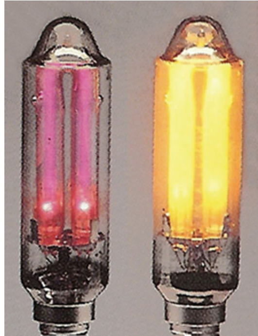
High- and Low-Pressure Sodium Lamp, Fig. 3 Immediately after switch-on, a low-pressure sodium lamp emits just a little reddish light, which gradually changes to the familiar yellow sodium light when the lamp has fully warmed up [1]
