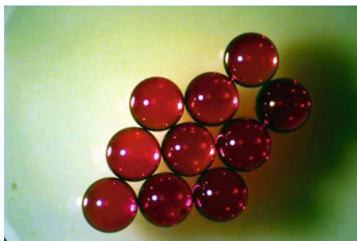
Transition-Metal Ion Colors, Fig. 1 Synthetic ruby spheres consisting of normally colorless \text{Al}_2\text{O}_3 doped with trace amounts of \text{Cr}^{3+}
