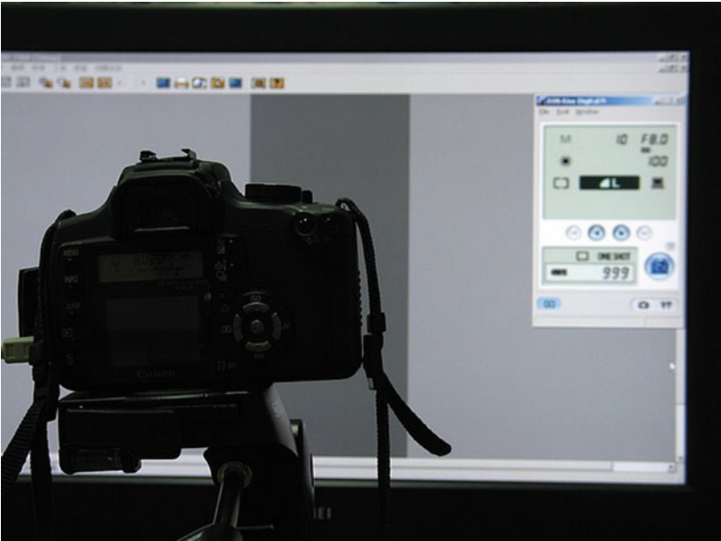
Luminance Meter, Fig. 1 Sharpness measurement of FPD by using a ILMD
