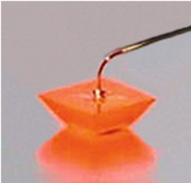
Light-Emitting Diode, LED, Fig. 7 An example of a specifically shaped LED chip that improves light-extraction efficiency. On top of the chip, the anode with its bond wire can be seen [1]
