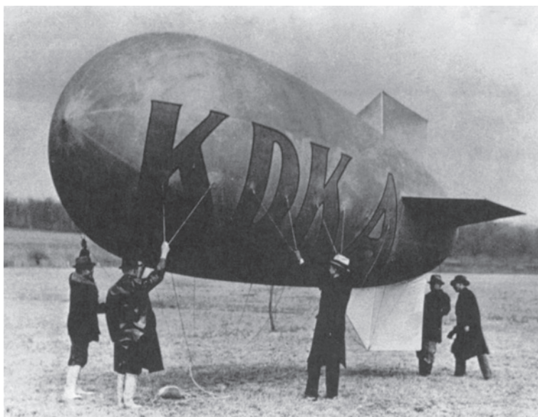
FIGURE 7.3 Station promotion in the early 1920s with an airborne antenna. Courtesy Wesinghouse Electric.
