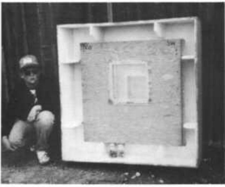
Fig. F.3. The Top and Four Walls of the Multi-Purpose Emergency Exit Housing, Nested Together to Save Storage Space. (Photograph)
