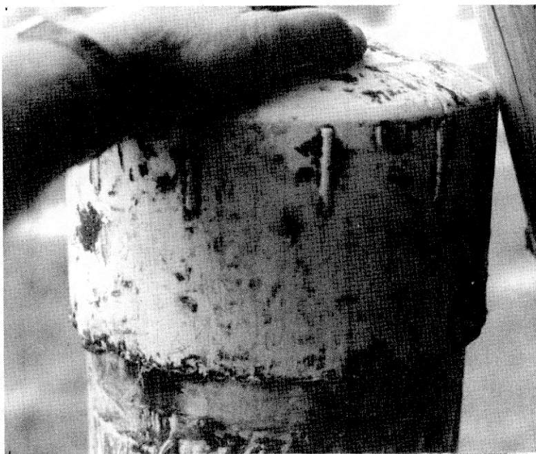
Placing slip cap onto cache tube.
