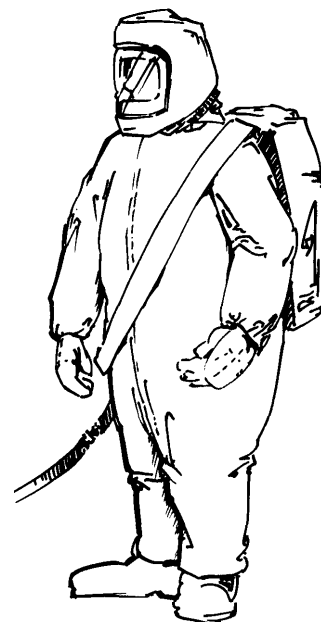
A fully encapsulating suit is generally the required dress for response personnel in incidents involving toxic substances. These suits are extremely bulky and cumbersome, and provide only half an hour of actual intervention time.
