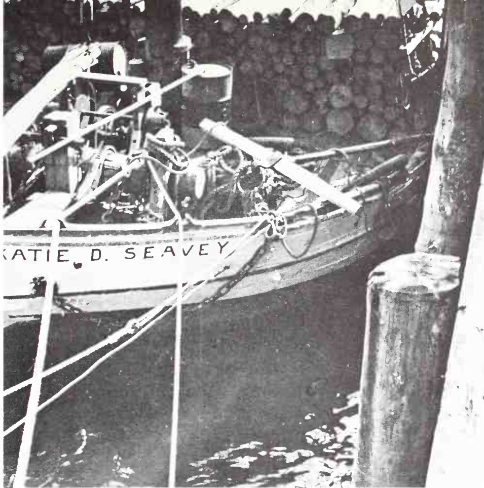
A dockside view of Katie D. Seavey showing the deck cargo reaching almost to the sidelights in the rigging. Just enough space has been left at the bow to work her windlass and handle the anchors.
