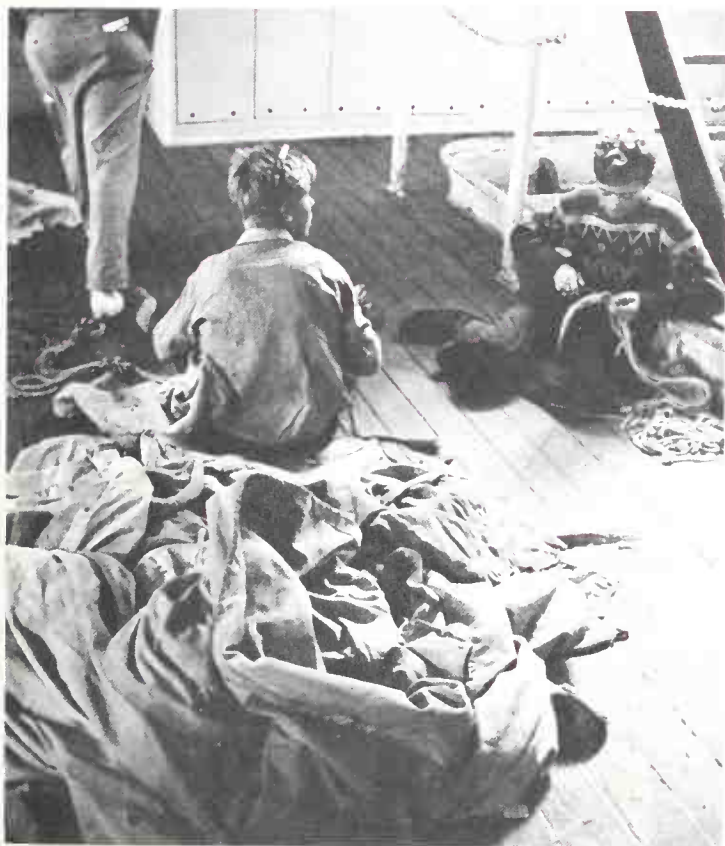
Old rope is unlaidd in the sail locker, the yarns to be used later as "baggy wrinkle" aloft to keep the stays from chafing against canvas.
