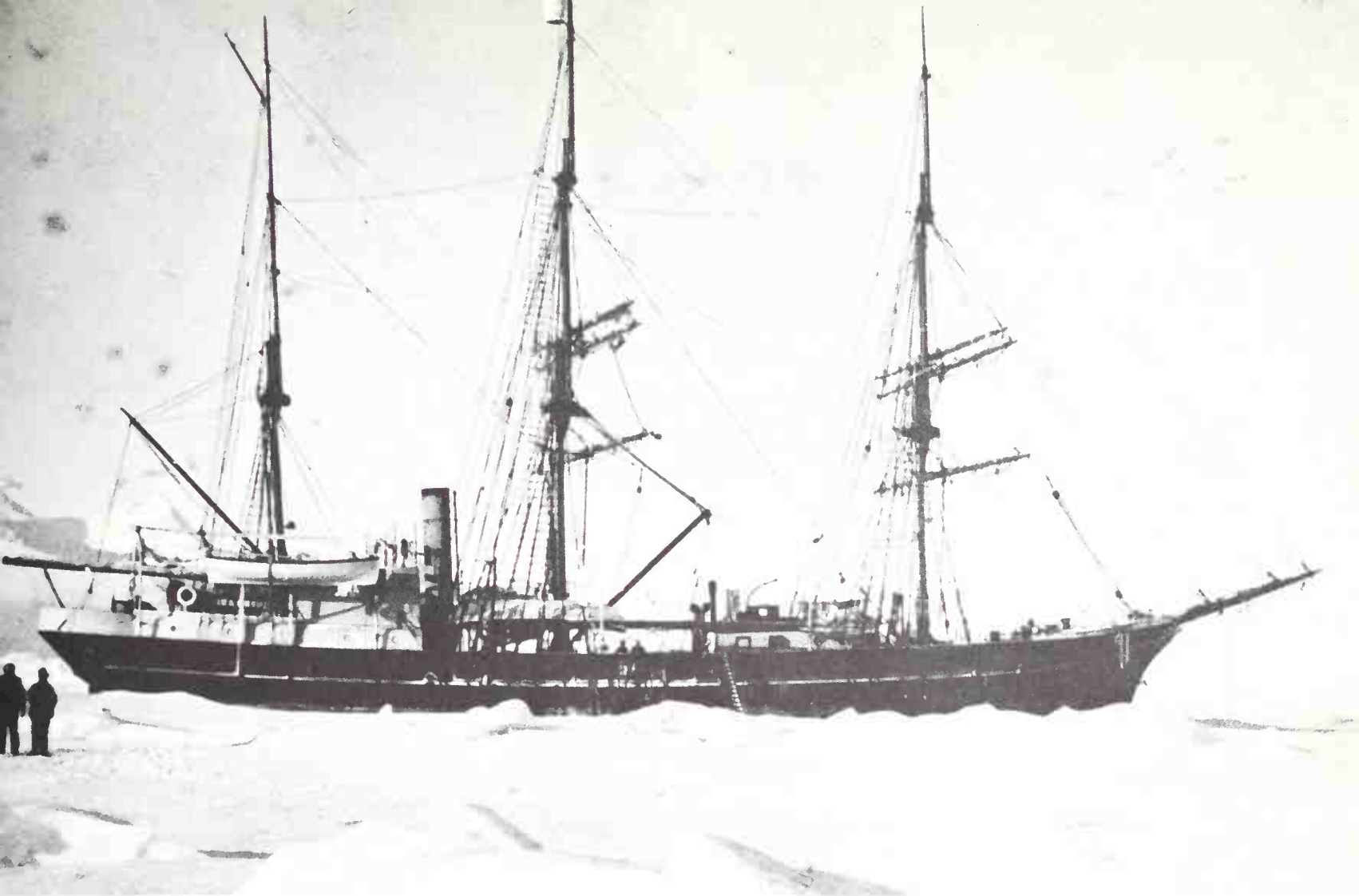
Typical of transition vessels, the steamer bark Scotia was built at Drammen, Norway in 1872 and used in Arctic explorations. She was destroyed by fire in 1916.
