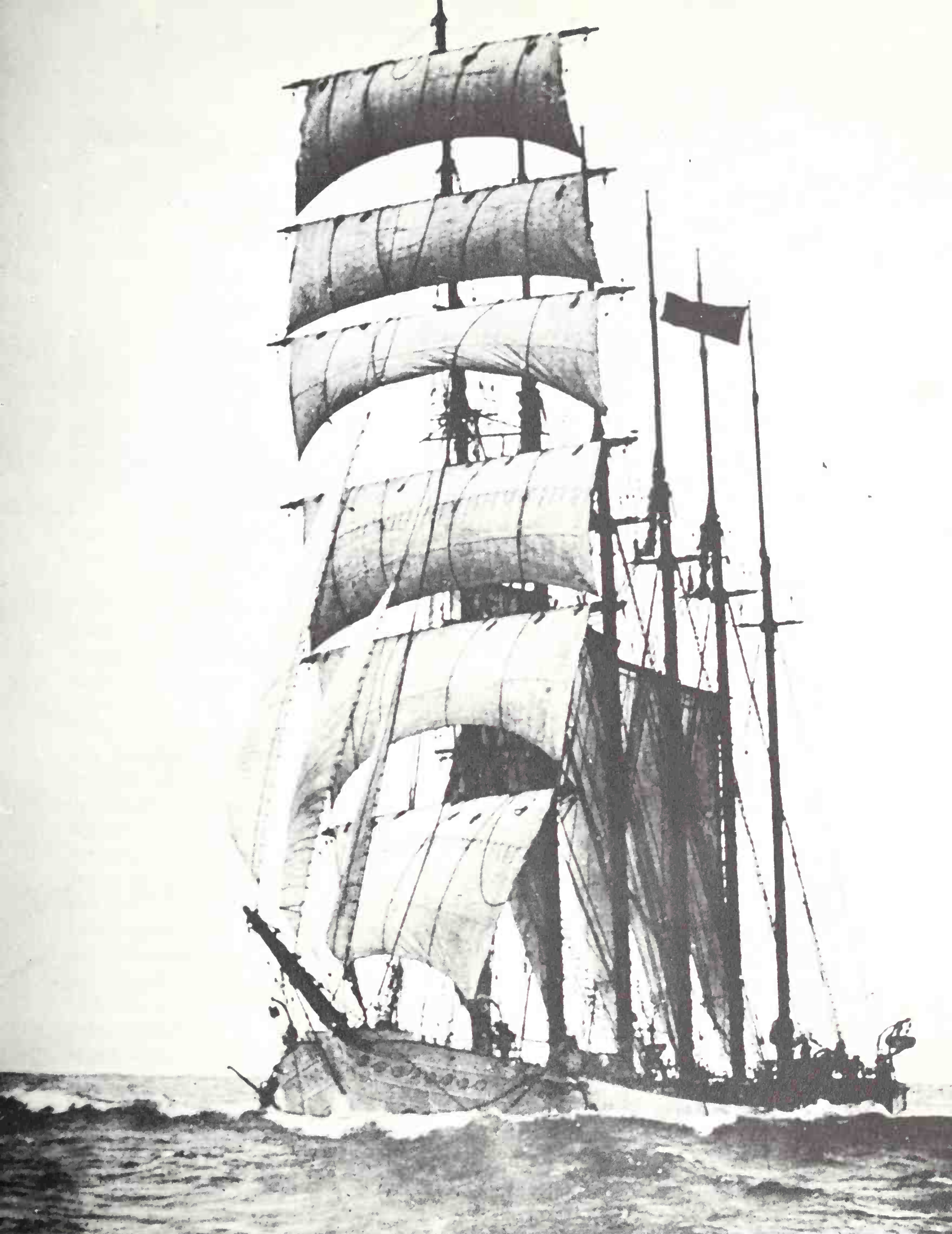
To survive the bitter competition with steamers, square-rigger men had to take chances. The Everett C. Griggs , renamed the E.R. Sterling , is loaded to the danger point. Both anchors are awash and she is taking water aboard in a fairly quiet sea.
