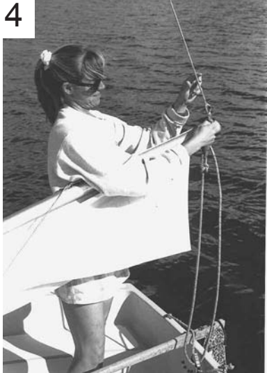
Unclasp the main halyard (rope that pulls up the main sail) from the boom.
