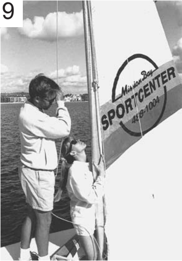
Haul up the mainsail, making sure the mainsheet is uncleated.
