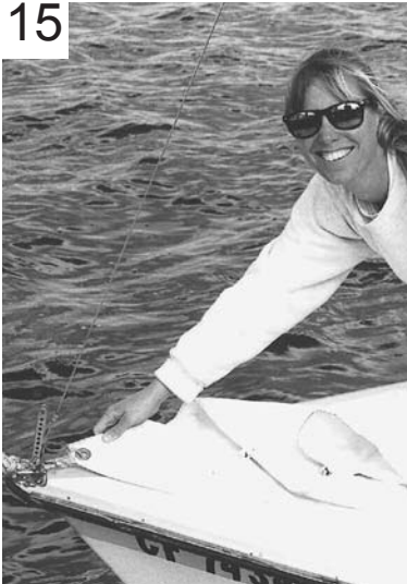
Hook bottom of jib to bow.
