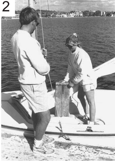
Slide in the daggerboard.
