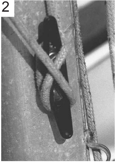
Cleat knot — For cleating the halyard.
