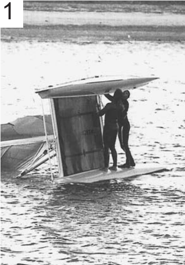
Capsize recovery — After releasing the sheets, Cliff tosses the righting rope over the upended hull ...
