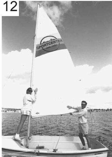
Check for sagging along boom and mast.
