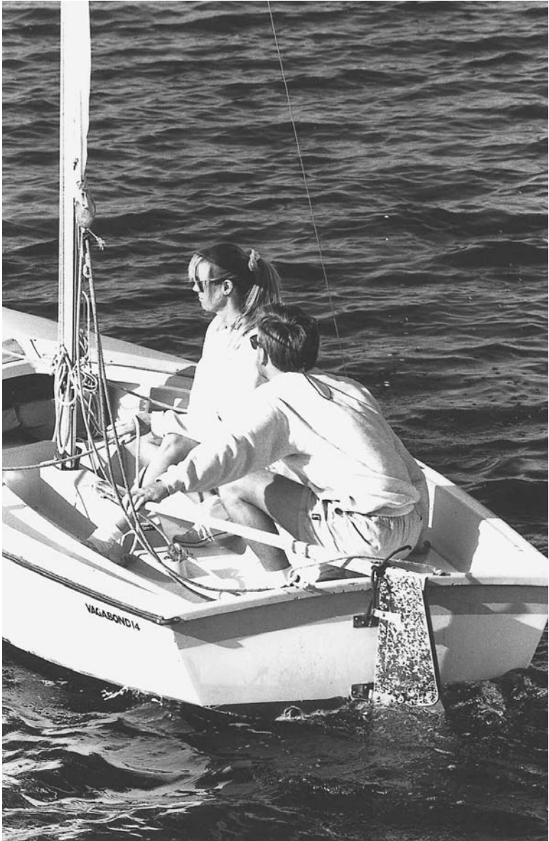
Beginning a tack — Cliff starts his turn from a closehauled course by pushing the tiller away.
