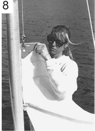
Slide mainsail into the slot on the mast.
