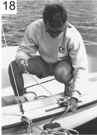
... and through their respective cleats. Tie ends in figure-eight knots. See page 91 for knot. Do not cleat.
