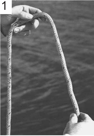
Bowline — For attaching a line to anything. It does not slip.
