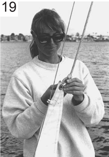
Attach jib halyard to top of jib.
