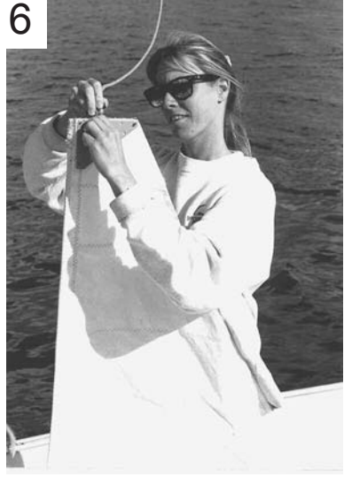
Attach main halyard to top of mast.
