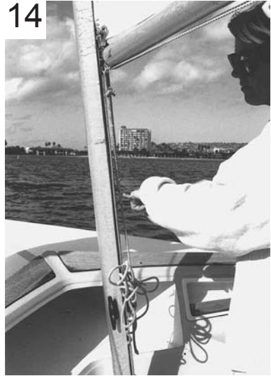
Adjust downhaul for sagging along the mast.
