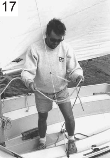
Jib sheets go around the shrouds (wires holding up mast) ...
