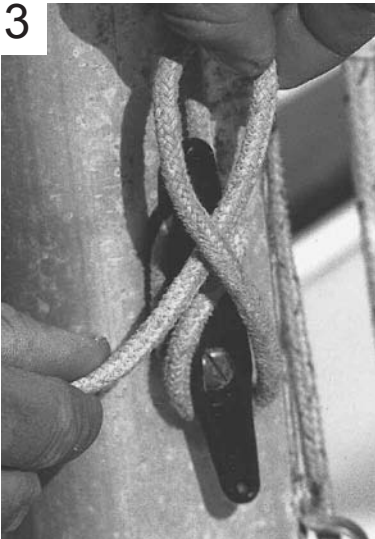
Cleat knot — For cleating the halyard.
