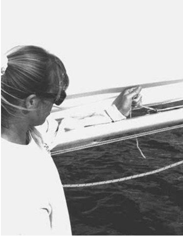
Adjust outhaul for sagging along the boom.
