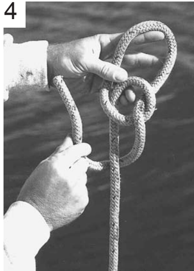
Bowline — For attaching a line to anything. It does not slip.
