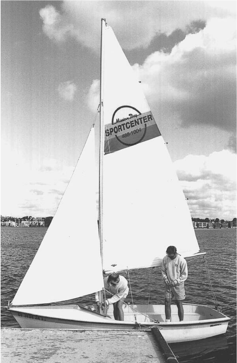
Check it out — Step back and take a look. Sails should be pulled all the way up and out. No sagging.
