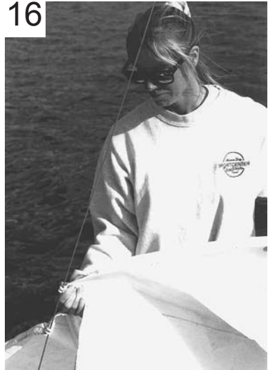
Fasten jib to forestay (the wire stretching from bow to top of mast).
