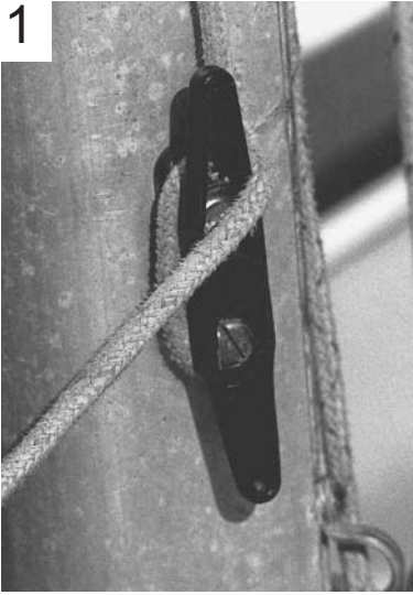
Cleat knot — For cleating the halyard.
