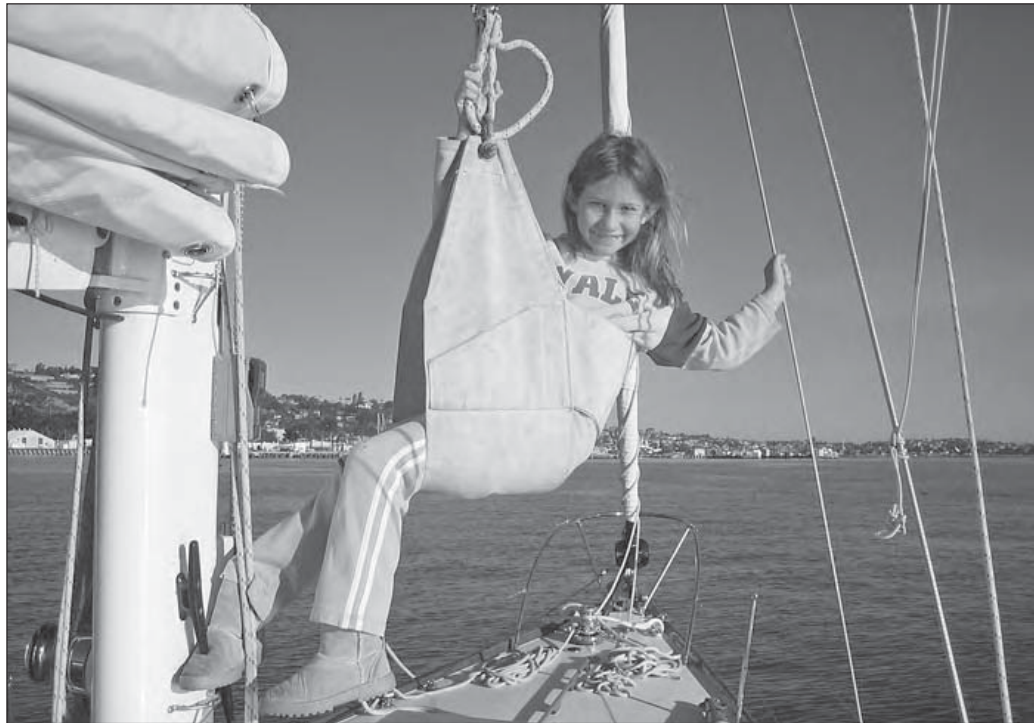
Figure 15-6: A bosun's chair provides comfort and safety when going up the mast.
