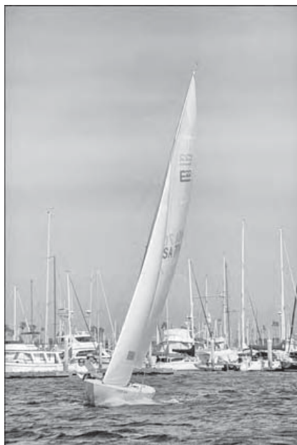
Figure 5-3: Sailing close- hauled with sails trimmed in tight.
