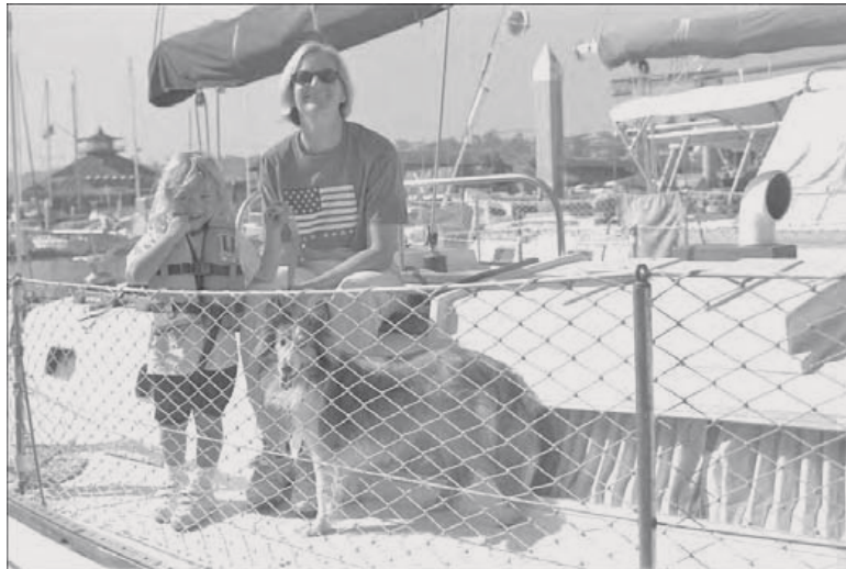
Figure 16-1: Weave netting onto the lifelines of your boat if you have a toddler onboard.
