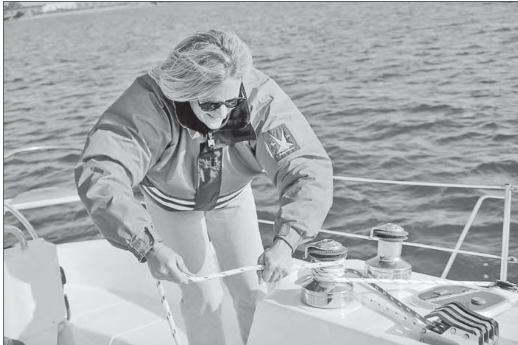
Figure 5-17: Keep pulling on the line as you use both hands to add a wrap on a highly loaded winch.
