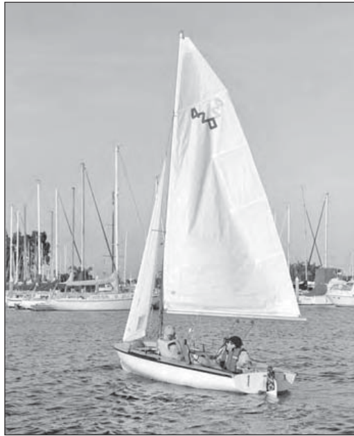
Figure 14-3: Heaving-to: Cleave the jib on the windward side and let the main luff. Now you can take a break.
