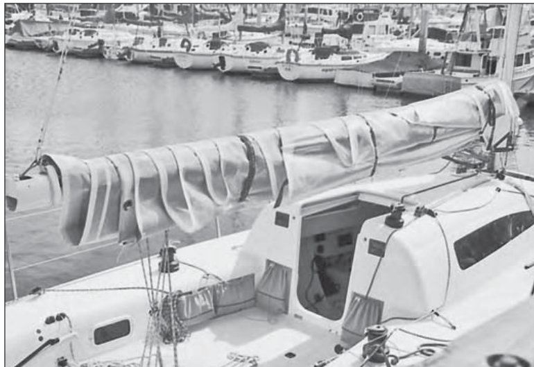
Figure 15-7: A mainsail flaked on the boom and secured with ropes or sail ties.
