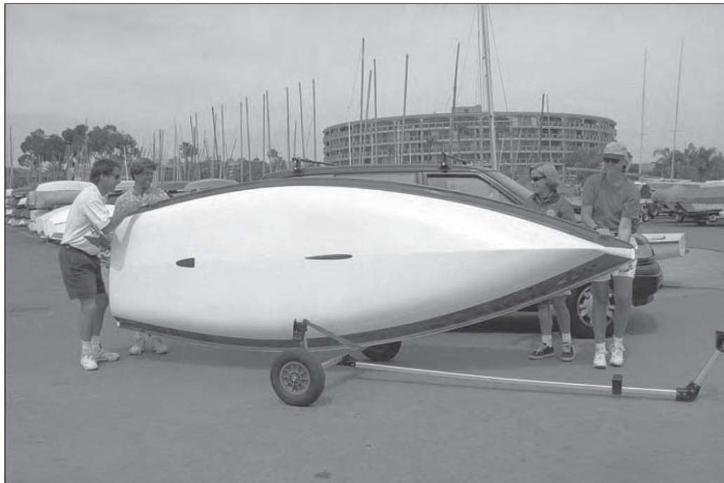
Figure 6-8: As you flip your boat, always make sure to set it on padding to protect the hull.
