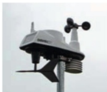
Below: The Vantage Vue system enabled us to record wind speed every second
