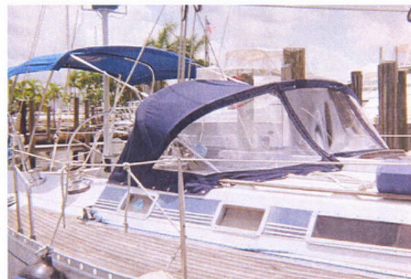
Dodger A demountable cover rigged over the companionway and the forward end of the cockpit to protect the crew from wind and water spray.
