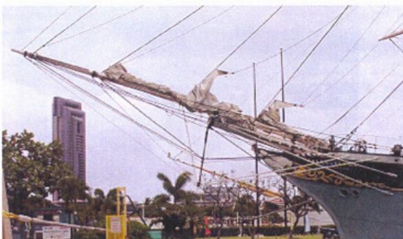
Bowsprit A spar which projects from the bow of some boats to allow headsails to be secured further forward.
