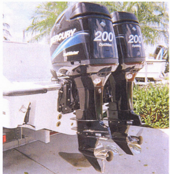
Typical Twin Outboard motor set-up.
