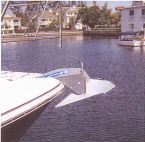
Anchor: A device attached to rope or chain which is lowered to the seabed to hold a vessel in place.
