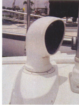
Ventilators: Movable devices fixed to the deck to carry fresh air below without permitting the entry of water. These are found both on power and sailing vessels.
