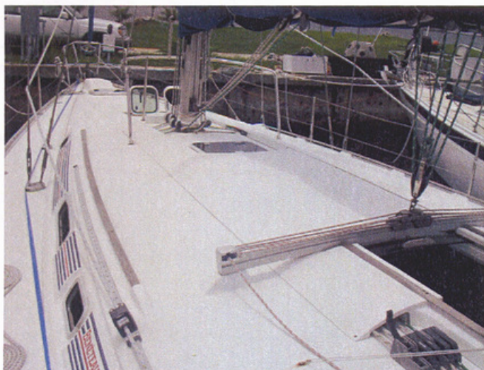
Coach Roof The raised part of the deck to create headroom below decks.
