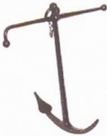
Fisherman/Admiralty The traditional type of anchor is sometimes known as an Admiralty Pattern anchor.
