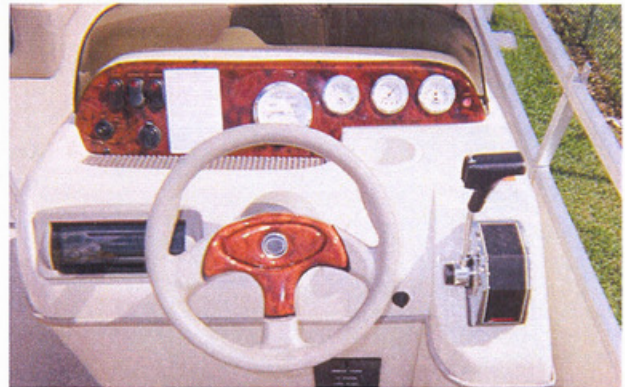
Console: Steering console, instrumentation and throttle control
