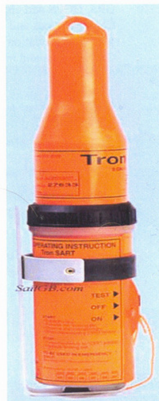
SART Search And Rescue Transponder 3 cm radar band
