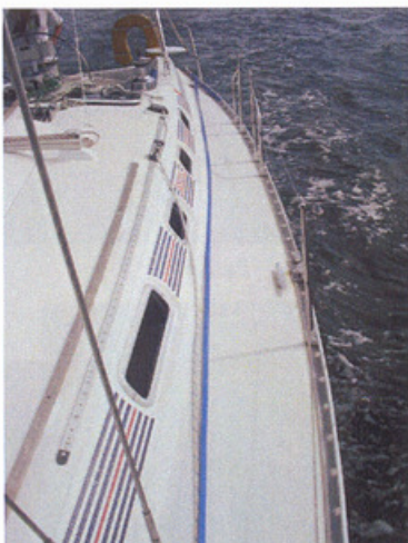
Jackstay A wire or webbing strap attached at the front and back of a vessel along the deck to which a safety harness line may be clipped. (mostly found on sailboats)
