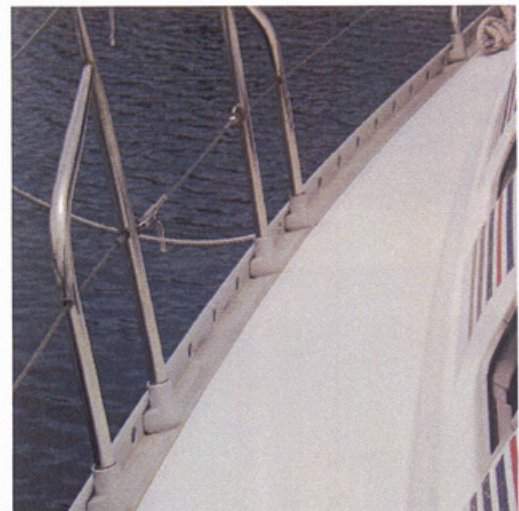
Toe rail A low timber or metal strip running around the outer edge of the deck to assist the crew in maintaining a foothold.
