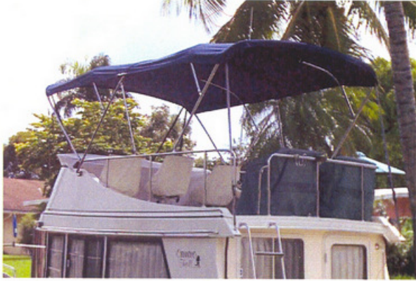
Bimini Top: A canvas canopy to shade an area of deck or cockpit from the sun.
