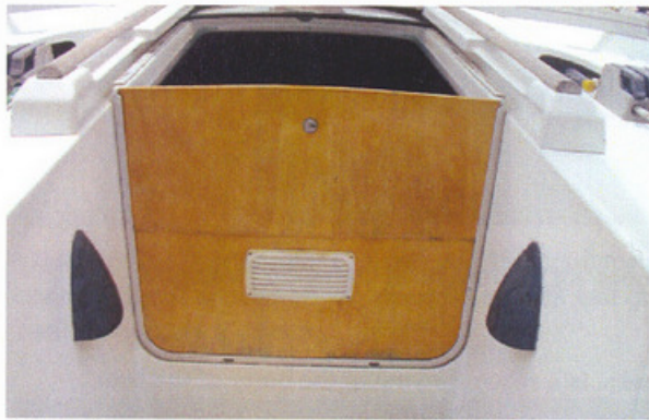
Washboards Boards used to seal off the companionway to prevent the entry of water.
