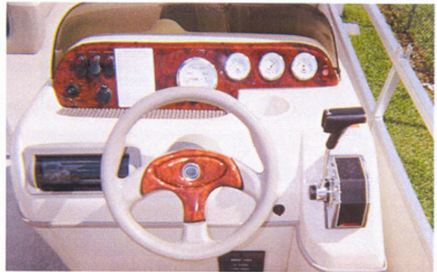
Console: Steering console, instrumentation and throttle control
