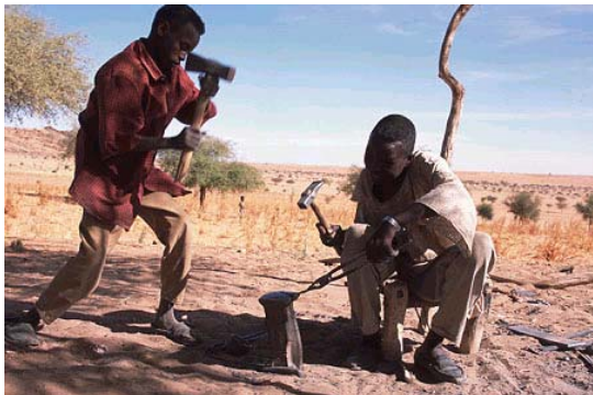
Figure 4: hammering one of the component parts of the plough ©Practical Action
