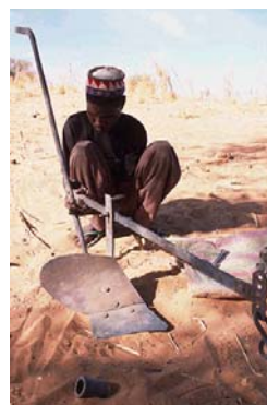
Figure 6: Assembly of the plough ©Practical Action
