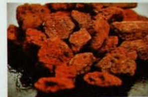
Lava rock, washed clean, is an excellent bio-filter medium.
