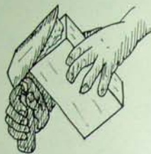
6. Butter brick end with sharp downward motion.
