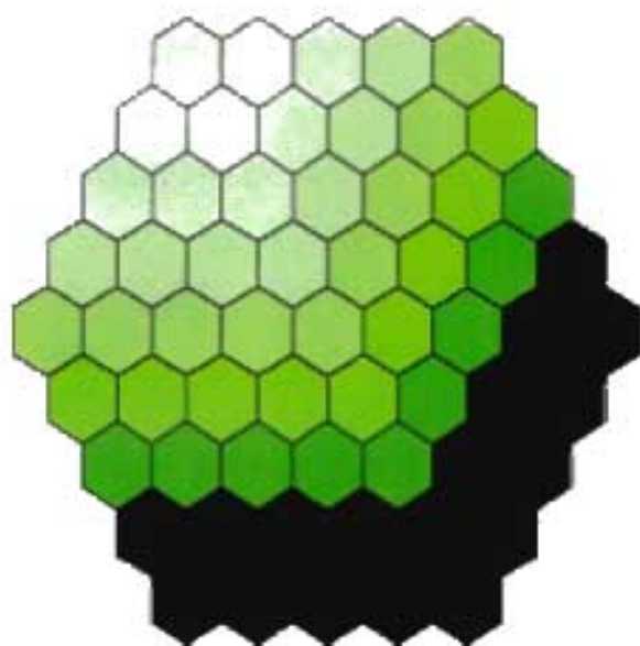
Figure 2.6 Hexagons are symmetrical in all diagonal flows and are convenient when describing dispersion.
