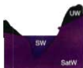
Figure 6.21 How water can re-emerge from the saturated layer and return to the surface water flow
