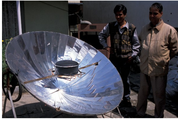
Figure 3: A solar parabolic cooker being used in Nepal ©Practical Action/N. Bruce
