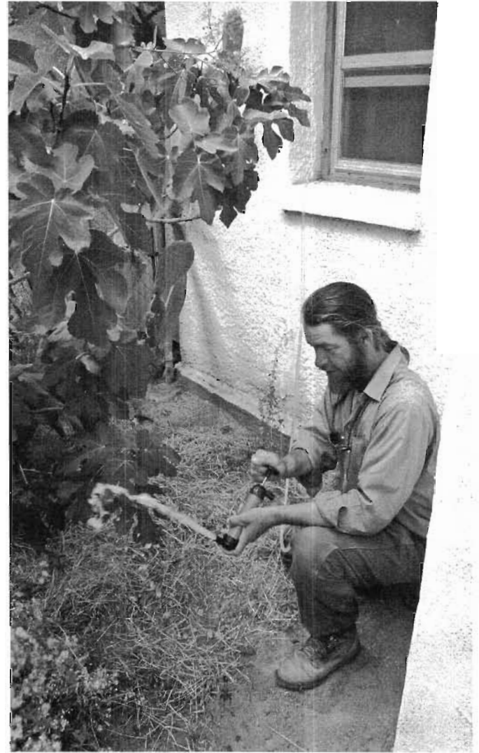
Fig. 4.28B. Siphon hand pump (from auto parts store) pulls tub greywater through tube. Once the water is flowing the pump is pulled off, the tube is placed beside the fig tree, and the siphon effect continues to draw the water. Buy the tube after the pump so you can size the tube diameter to fit the pump. See volume 2 for other variations.
