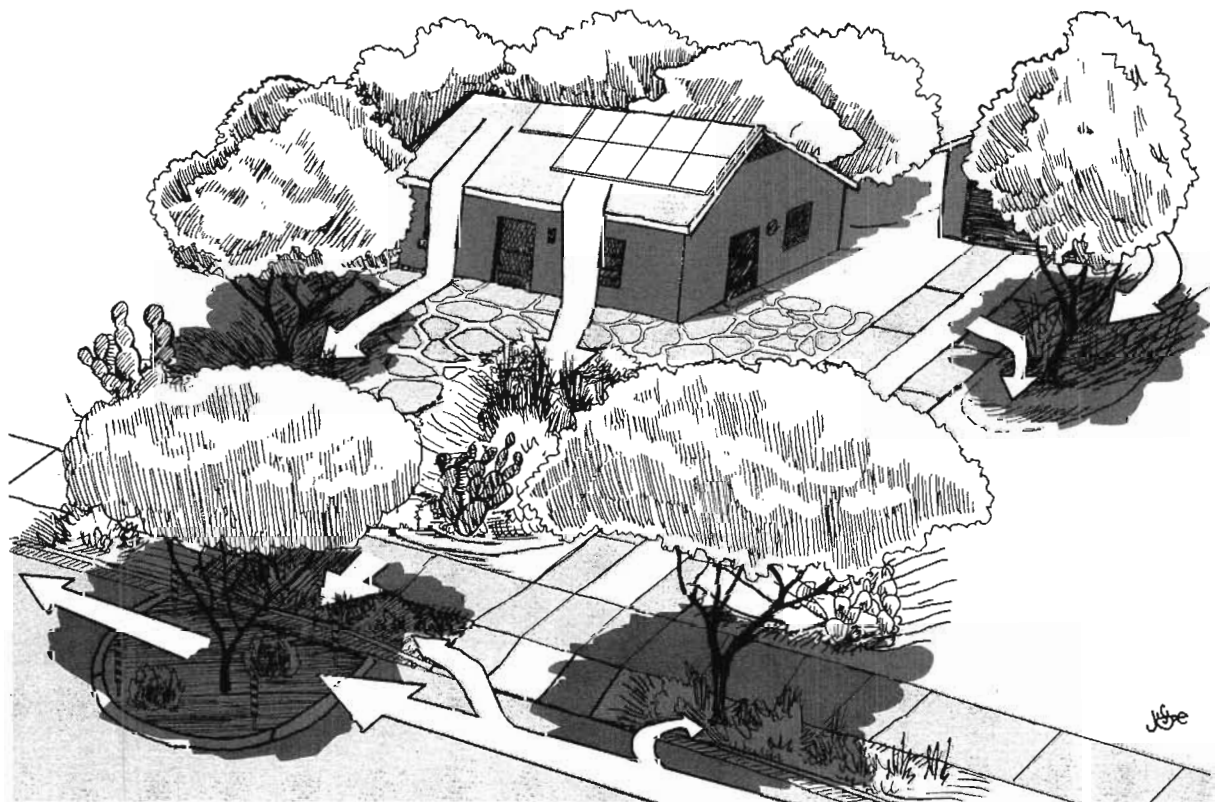
Fig. 4.18B. A hydrated and sheltered residential lot dominated by water-harvesting earthworks, native low-water-use vegetation, and permeable paving graded to minimize runoff and utilize it on-site.
