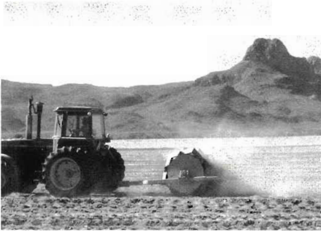
Fig. 3.13A. An imprinter roller pulled by a tractor creating and seeding imprints on barren, compacted earth, Marana, Arizona
