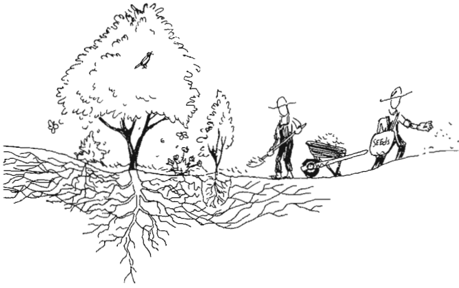
Fig. 1.18. Planting vegetative groundcover, spreading organic mulch, and planting seed to help permeate, protect, and build soil with roots, leafy cover, mulch, and accumulating leaf drop
