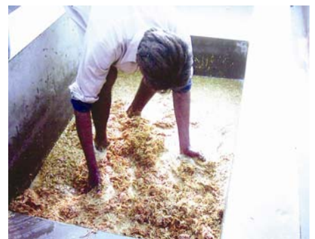
Figure 8, 9. Add soaked wheat straw to the lime stone solution
