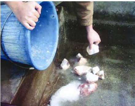
Figure 4, 5, 6. Add lime stones to the other container and they dissolve emitting heat and gas
