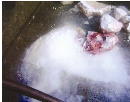
Figure 4, 5, 6. Add lime stones to the other container and they dissolve emitting heat and gas
