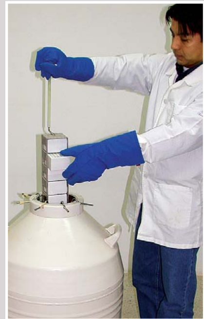
Figure 4. Vials placed in polycarbonate containers directly frozen in liquid nitrogen
